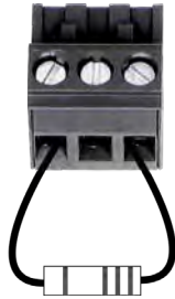
Figure B.2.22 – Terminating the Amplifier Input
