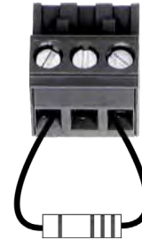
Figure B.2.39 – Terminating the Amplifier Input
