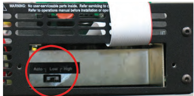
Figure 6.12 – Bi-Level Power Switch Location
