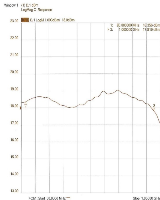
Figure 4-4. Typical Module Response
