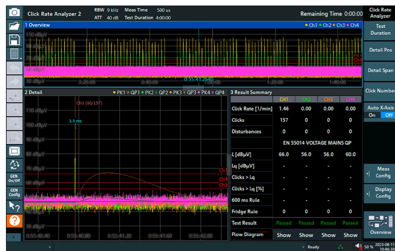
Analysis of the emissions of an oven using the R&S®EPL1-K59 click rate analyzer option. Clicks are identified on CH1. The complete timeline at the top shows a nearly regular distribution of the pulses. The detail window shows that the quasi-peak detector exceeds the limit. Although several clicks are detected, the oven has passed the test.
