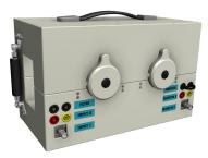
Coupling transformer for Cable Bundle testing used with WF1, WF2, WF3, WF5A, WF6. The CN-BT7 has a large aperture of  $6 \times 9 \text{cm}$  and is equipped with a monitor loop for calibration and supervision during the test.
