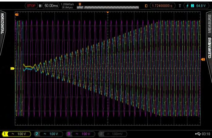
Figure 19: IEC 61000-4-34 Three Phase Voltage Variation Test
