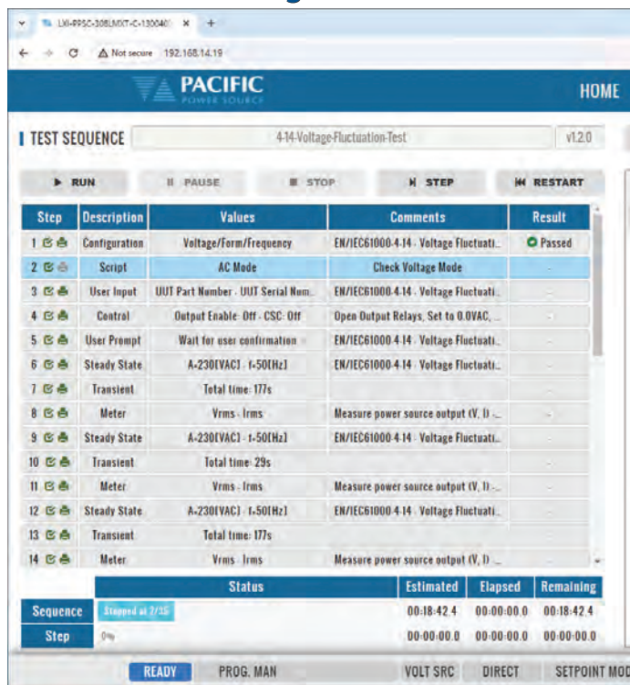
Figure 11: IEC 61000-4-14 Test Execution Control Screen
