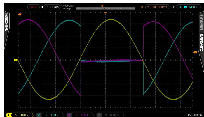
Figure 4: IEC 61000-4-11 1/2 Cycle Phase-to-Phase Voltage Dip
