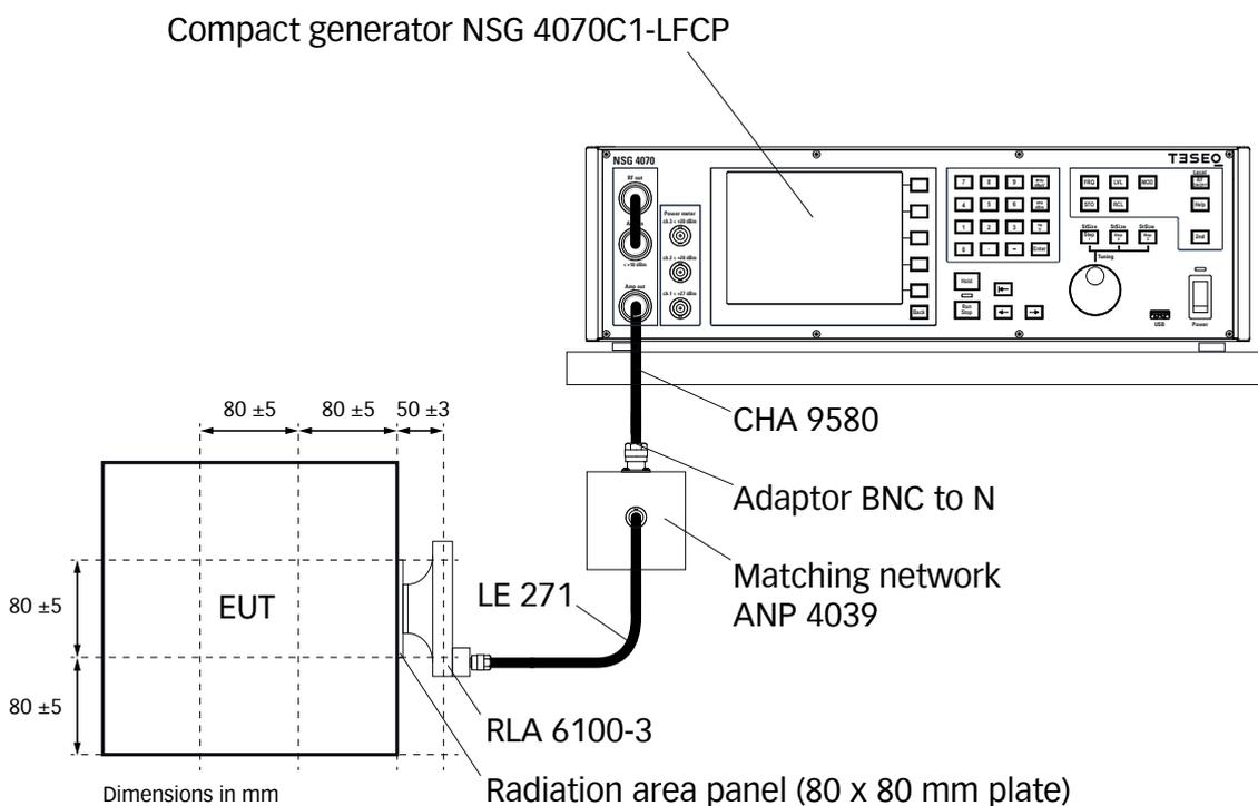
**Figure 4: Set up example for testing the frequency 13.56 MHz with ANP 4039**
