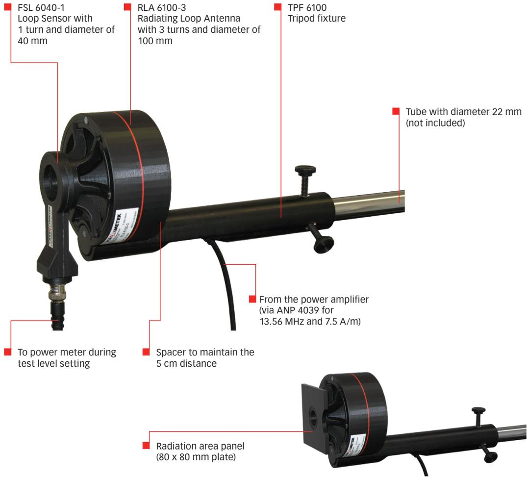
Figure 6: Construction of the product
