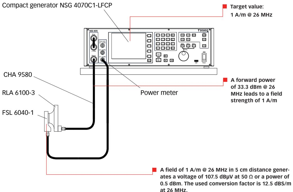
Figure 1: Set up example for test level setting for the whole frequency range
