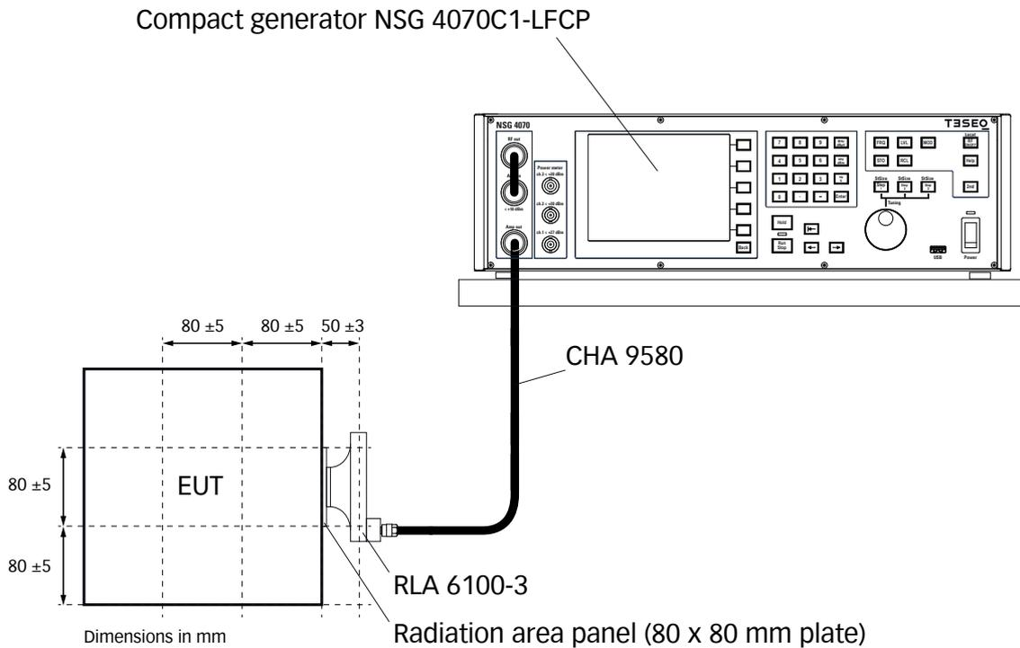
**Figure 3: Set up example for testing**
