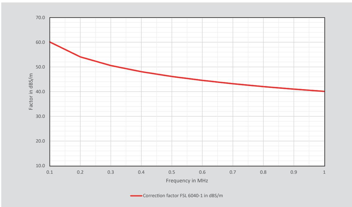
Figure 8: FSL 6040-1 Field Sensor Loop typical correction factor 100 kHz to 1 MHz
