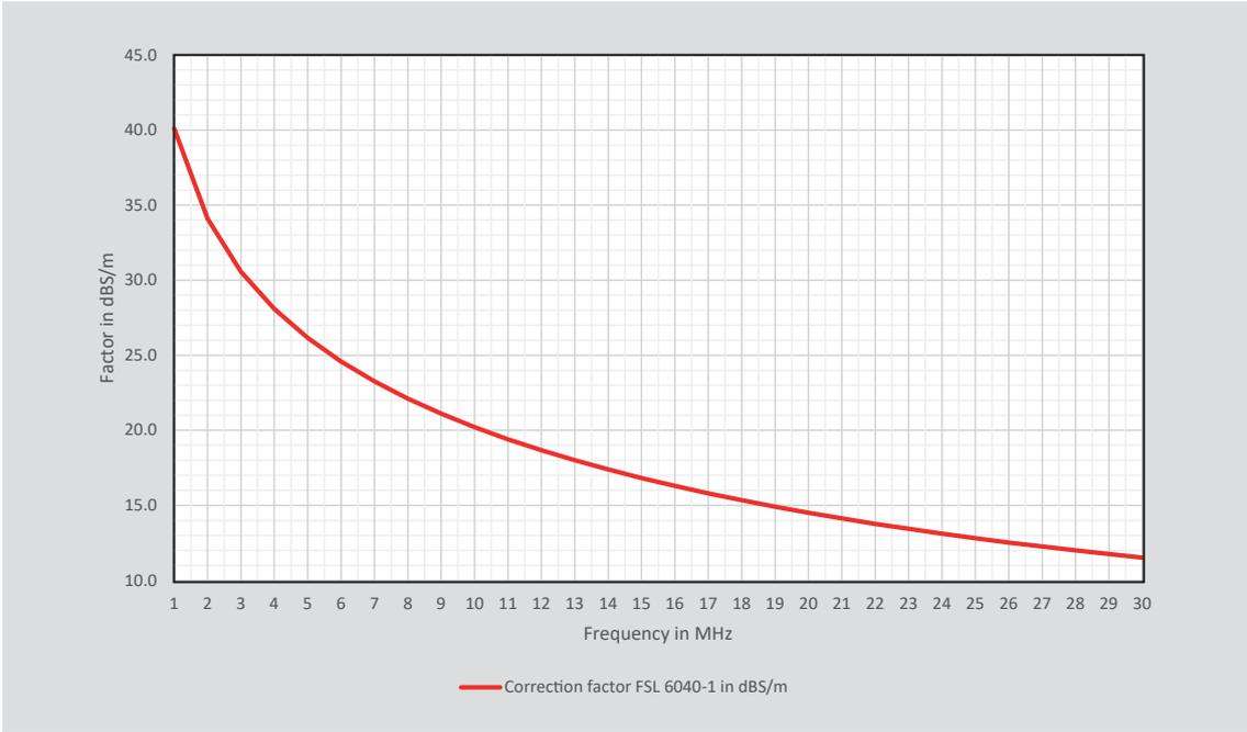
**Figure 9: FSL 6040-1 Field Sensor Loop typical correction factor 1 MHz to 30 MHz**
