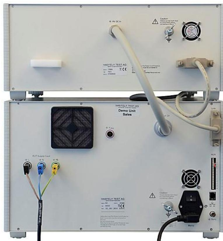
Figure 10-4: Connection AXOS 8 + TW 8 Module
