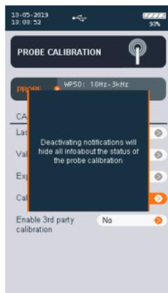
If the user chooses to use an external calibration, a new calibration date can be inserted and validity can be set by enabling 3rd party calibration.
