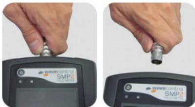
Figure 9: How to disconnect the field probe
