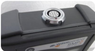
Figure 5: Push-pull connector
