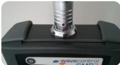
Figure 8: How to connect the field probe
