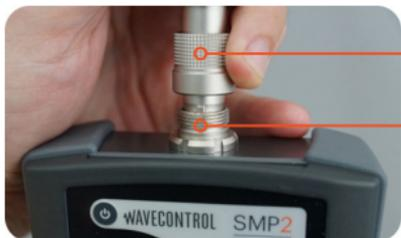
Figure 7: How to connect the field probe
