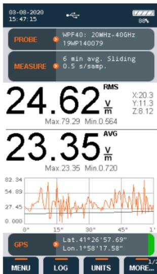
To start logging samples, press the 'LOG' button on the virtual menu. When logging starts, the device creates a new measurement record identified with its starting date.
