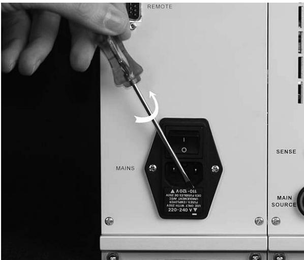
Picture 4-2: Loosen the drawer using a screwdriver.
