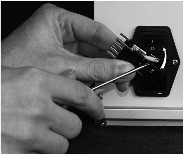
Picture 4-5: Remove defect fuses.
