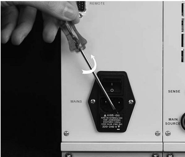
Picture 2-2: Loosen the drawer using a screwdriver
