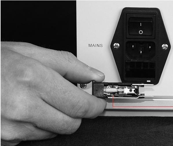
■ The defect fuse on the side of the drawer
