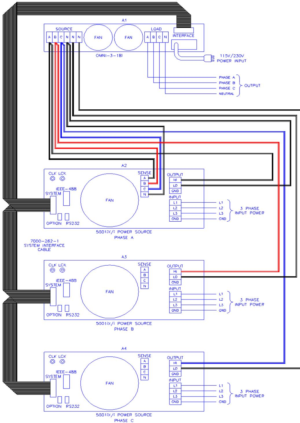
Figure 9-120: Schematic Showing Impedance 1-37i and 1-37iJ Connected to NSG 1007-5-208 System
