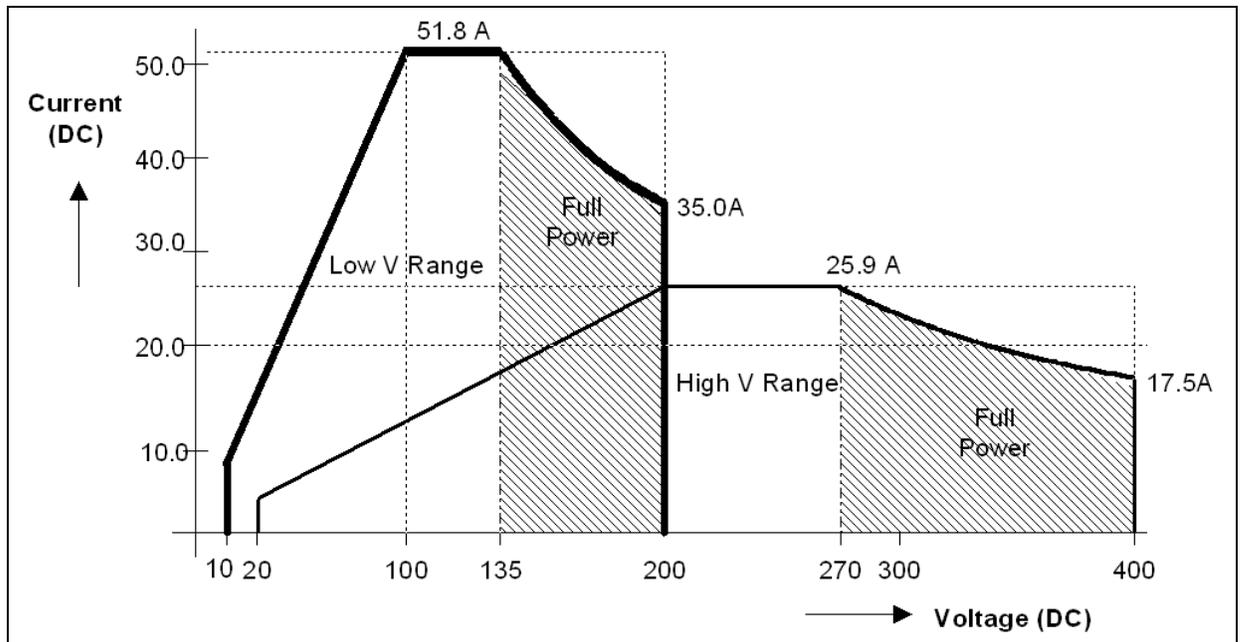
Figure 2-6: NSG 1007-10-208 / NSG 1007-30-208 - Voltage Current rating, DC mode
