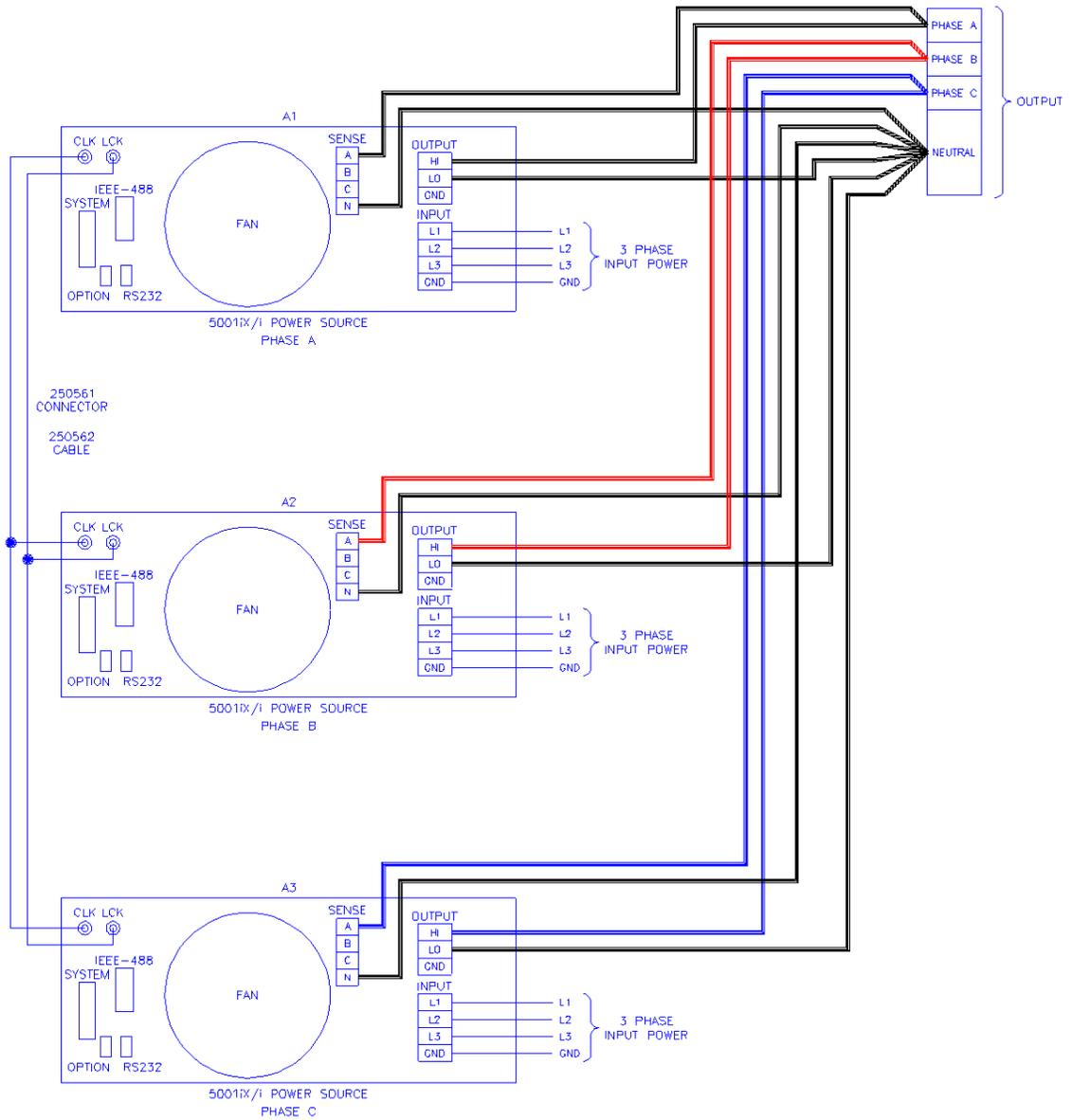
Figure 3-24: Single Phase 15000 VA System (NSG 1007-15S-208/i)
