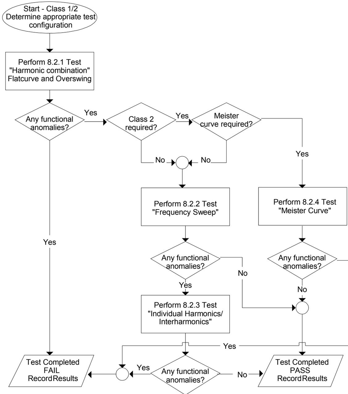
Figure 9-108: IEC 61000-4-13 Test Flowchart Class 1 and 2
