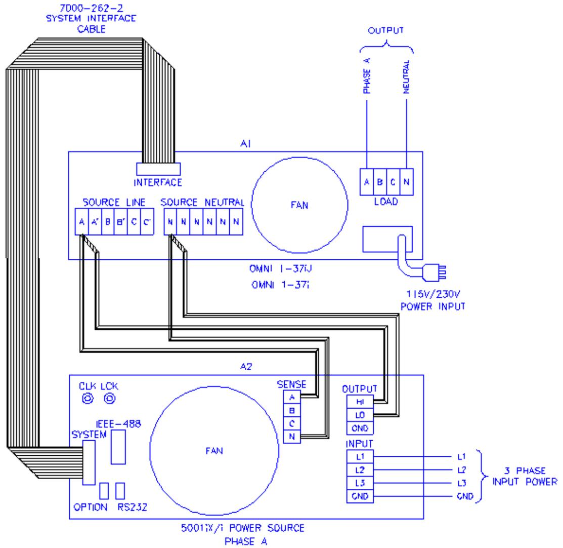
Figure 9-121: Schematic Showing INA 2153 Connected to NSG 1007-30-208 System
