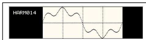
VIEW(F): This mode can be used to display any of the available user defined waveforms in a frequency domain display. Waveform data is shown by harmonic amplitude and phase relative to the fundamental frequency. Previewing a waveform can be useful if you are unsure about the nature of the waveform that was stored.
