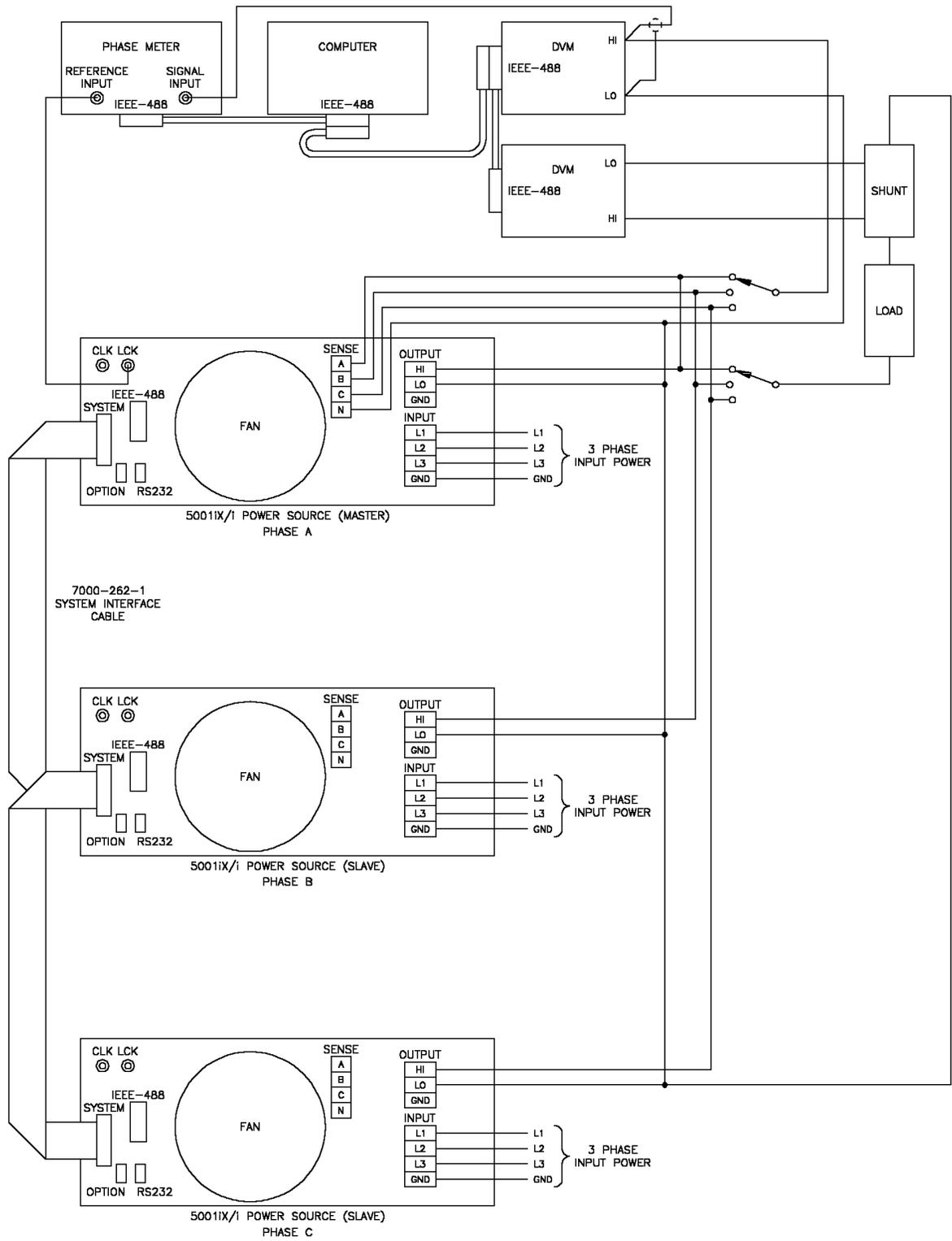
Figure 6-78: Test Equipment Hook-up for Measurement Calibration
