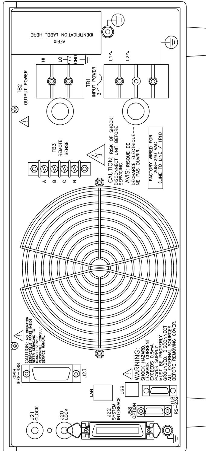
Figure 3-16: Rear Panel View for the 3001i/NSG 1007-3 (Series I, no USB)
