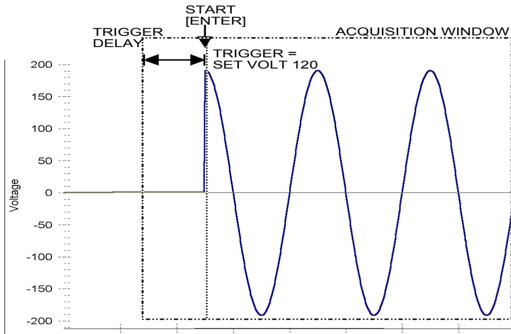
Figure 4-65: SET VOLT trigger source acquisition
