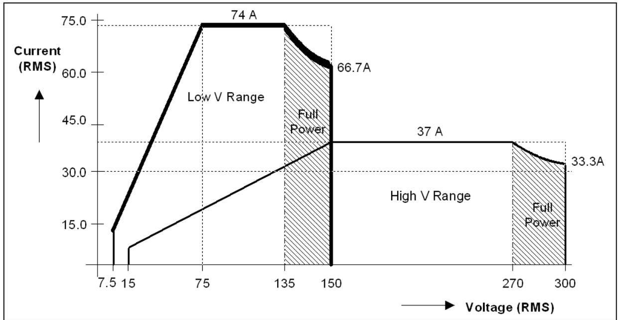
Figure 2-5: NSG 1007-10-208 / NSG 1007-30-208 - Voltage Current rating, AC mode
