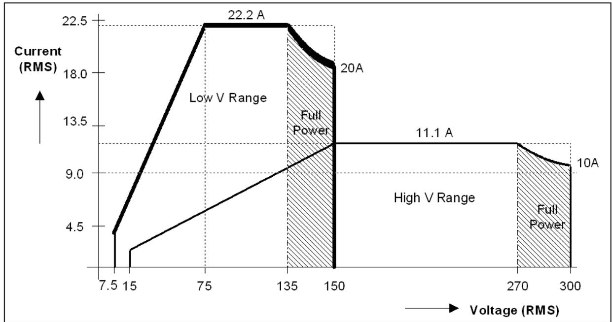
Figure 2-1: NSG 1007-3 / NSG 1007-9 - Voltage Current rating, AC mode
