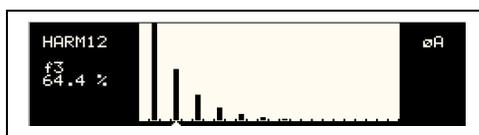
Figure 4-61: Waveform frequency domain view mode
