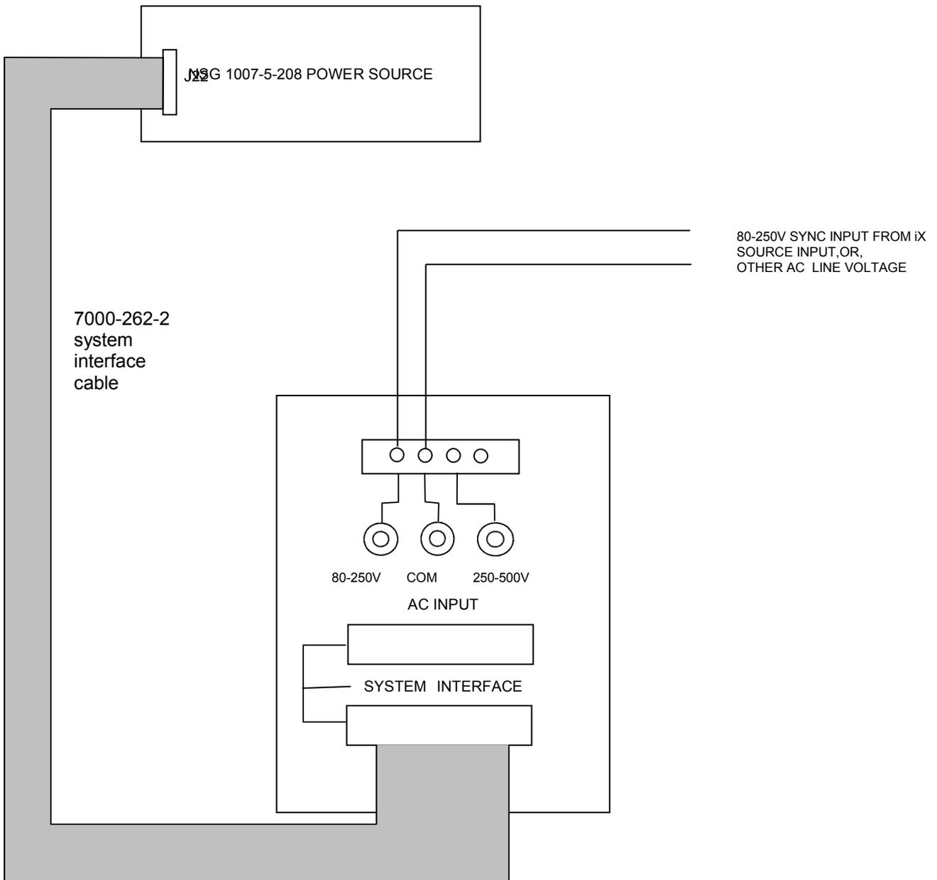
Figure 9-126: INA 2145 Connection on Low Range
