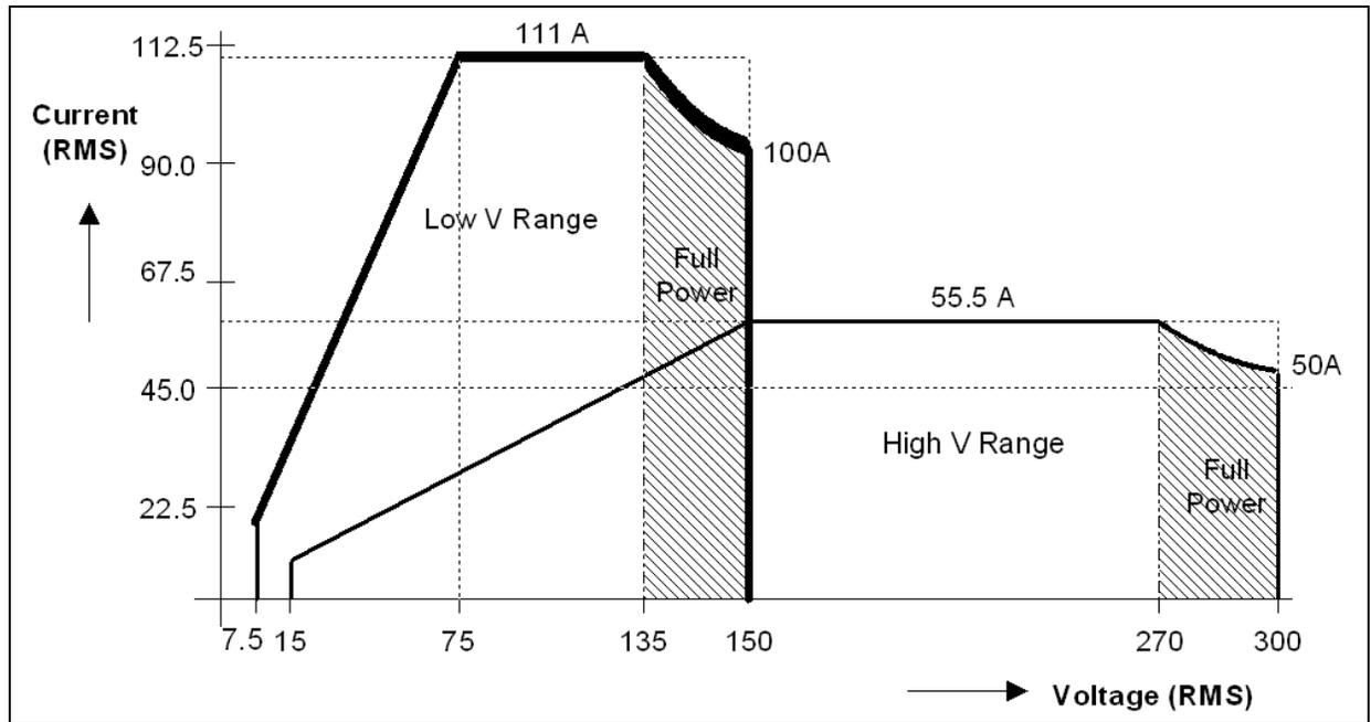
Figure 2-7: NSG 1007-15S-208 - Voltage Current rating, AC mode
