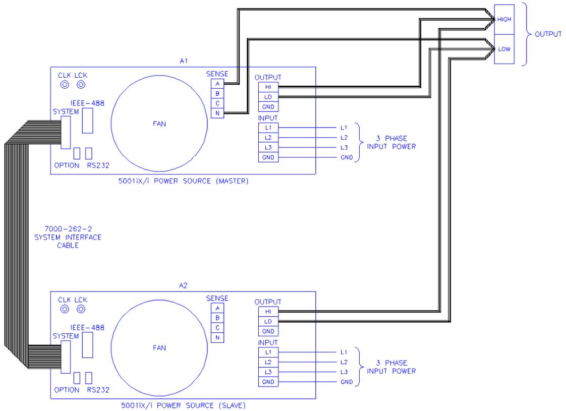
Figure 3-22: Two Phase 10000 VA System (10002i/iX – One Controller)
