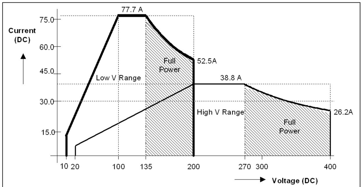
Figure 2-8: NSG 1007-15S-208 - Voltage Current rating, DC mode
