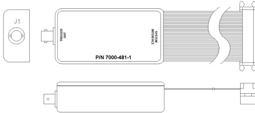
Figure 3-14: Function Strobe / Trigger Output Accessory.
