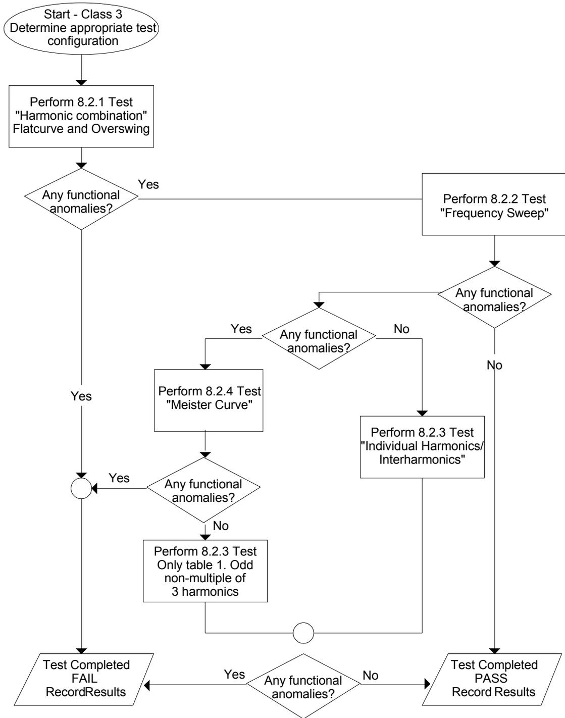
Figure 9-109: IEC 61000-4-13 Test Flowchart Class 3
