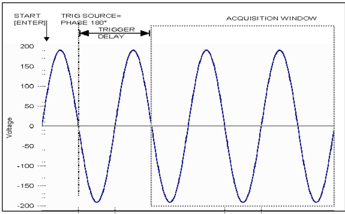
Figure 4-66: Positive trigger delay (Post trigger data)
