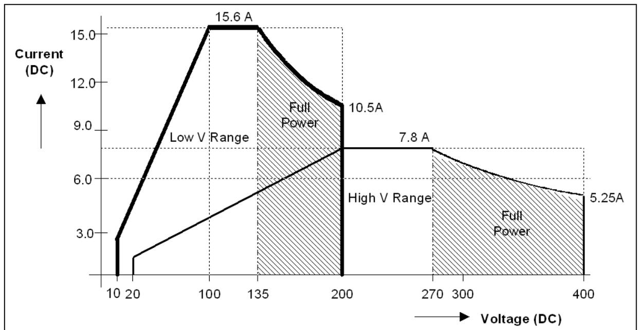
Figure 2-2: NSG 1007-3 / NSG 1007-9 - Voltage Current Rating, DC mode
