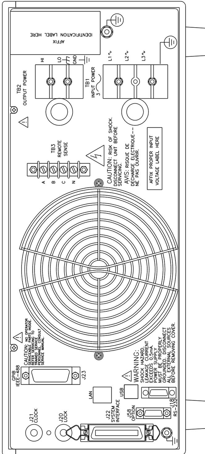
Figure 3-18: Rear Panel View for the 5001i/NSG 1007-5-208 (Series I, no USB)
