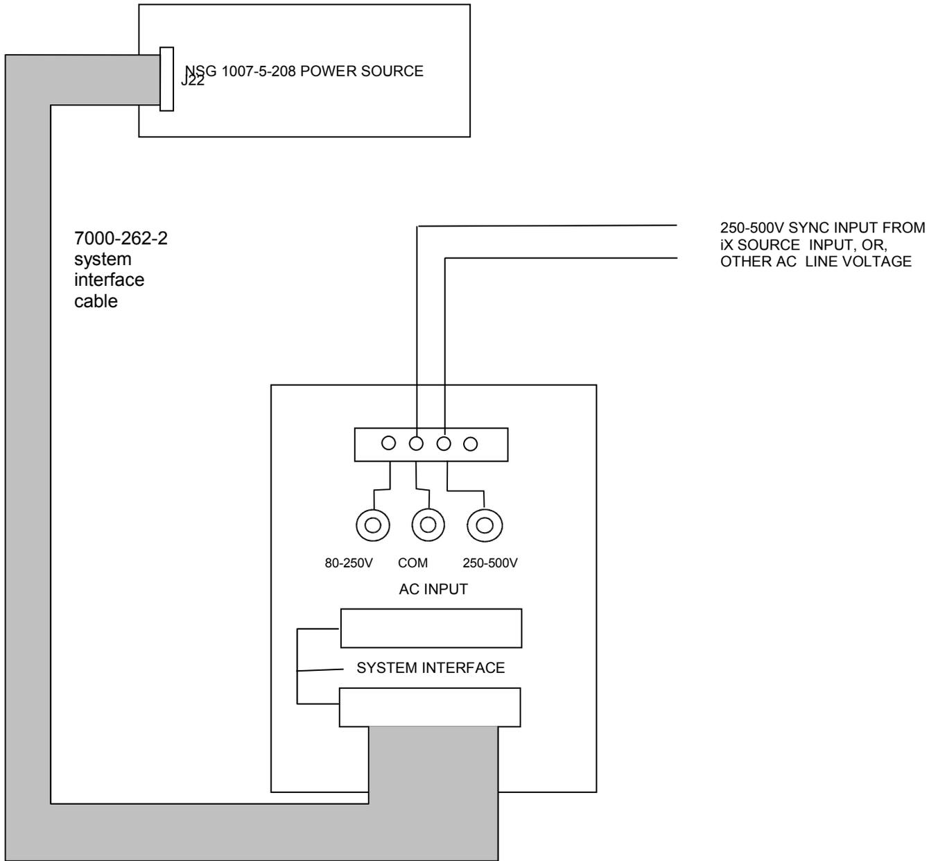
Figure 9-127: INA 2145 Connection on High Range
