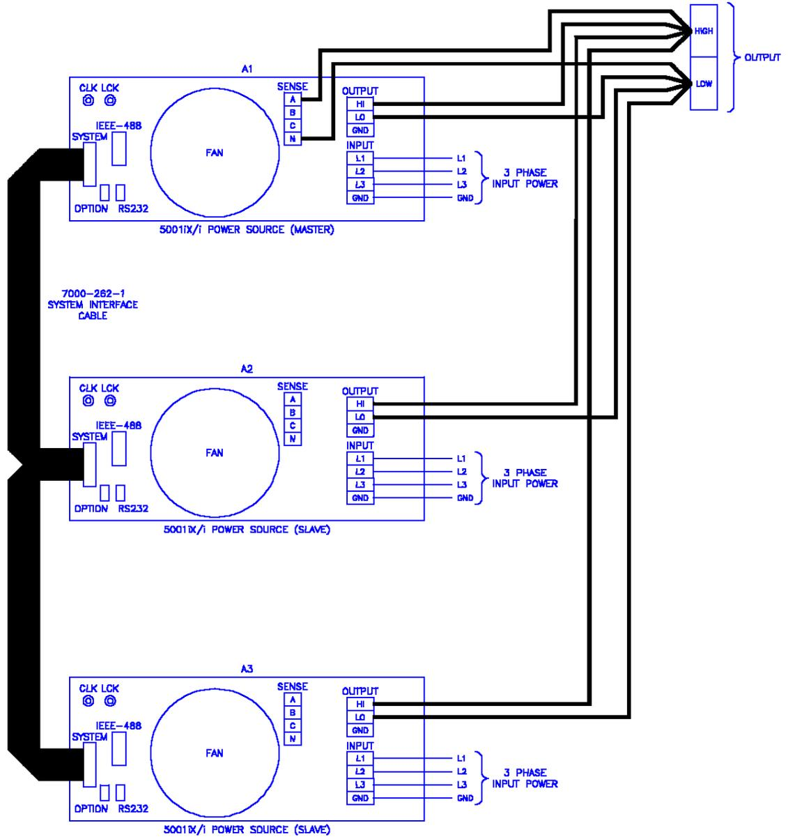
Figure 3-25: Three-Phase 15000 VA system (NSG 1007-15-208/i - One Controller)
