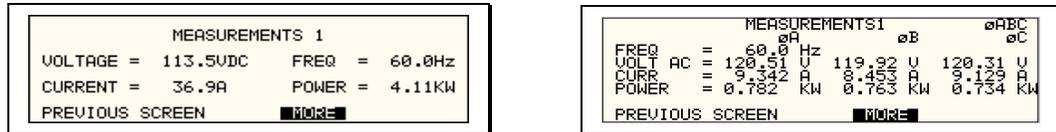
Figure 4-37: MEASUREMENTS Screen, single phase and three phase modes
