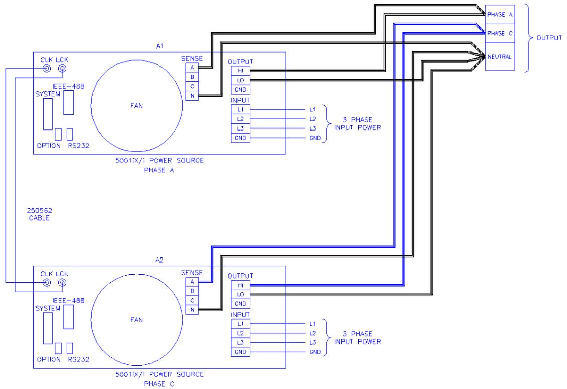
Figure 3-28: Three-Phase 9000 VA System (NSG 1007-9/i – One Controller)
