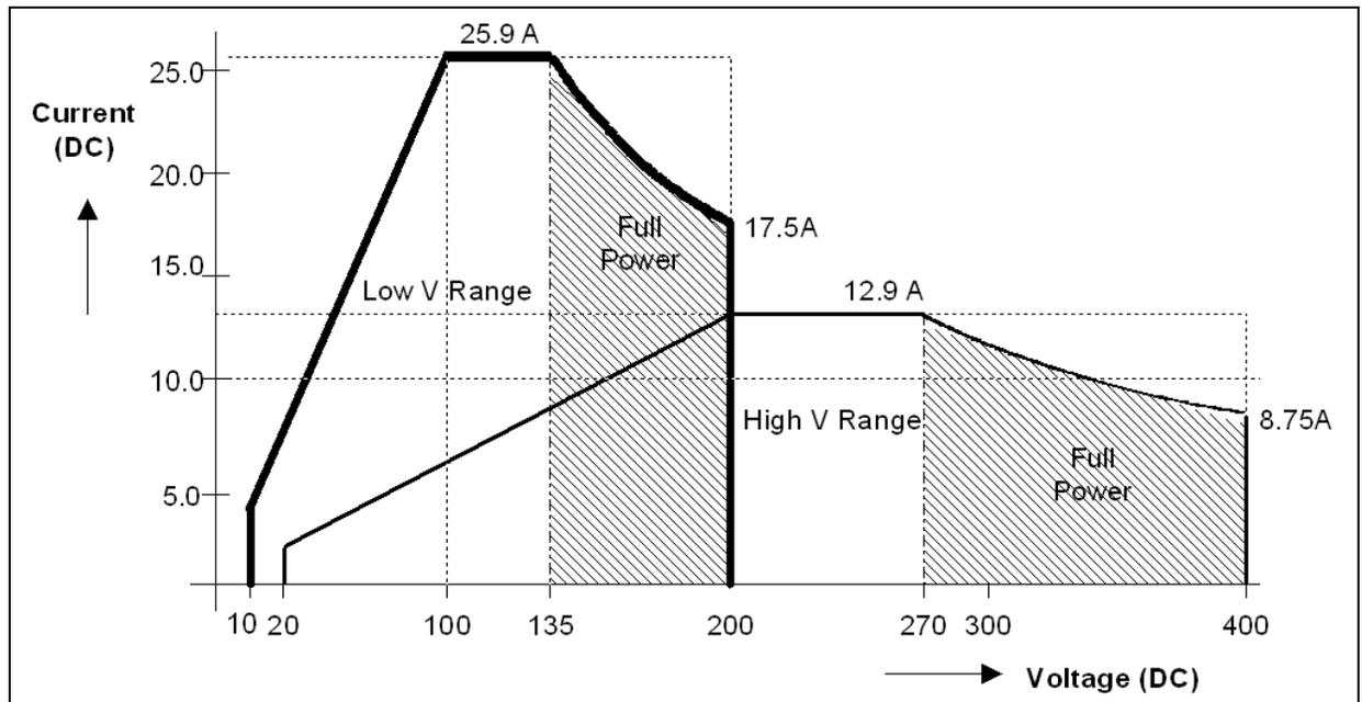
Figure 2-4: NSG 1007-5-208 / NSG 1007-15-208 - Voltage Current rating, DC mode
