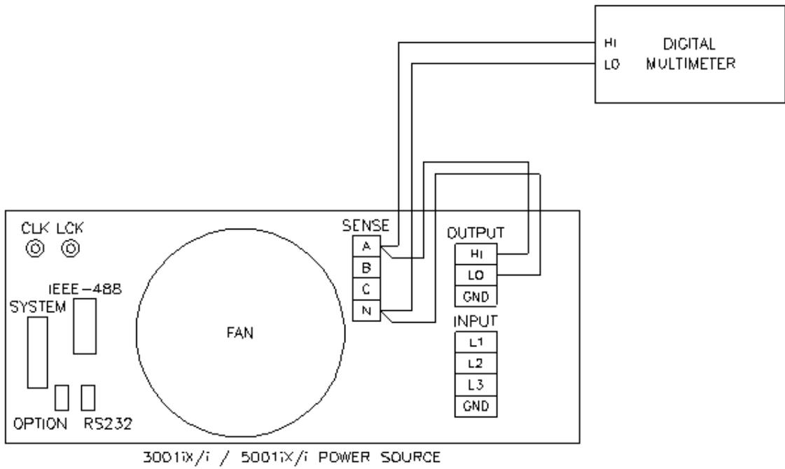
Figure 6-79: Test Equipment Hookup for Routine Output Calibration
