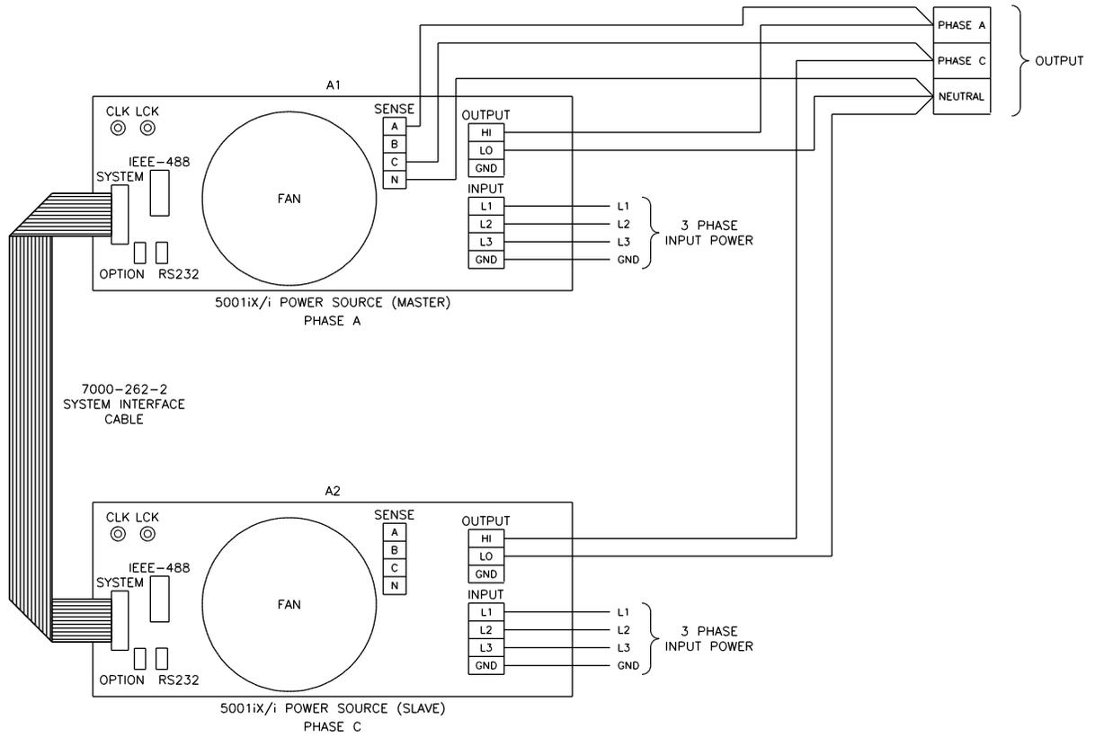
Figure 3-23: Three Phase 15000 VA System (NSG 1007-15-208/i-LK Three Controllers)
