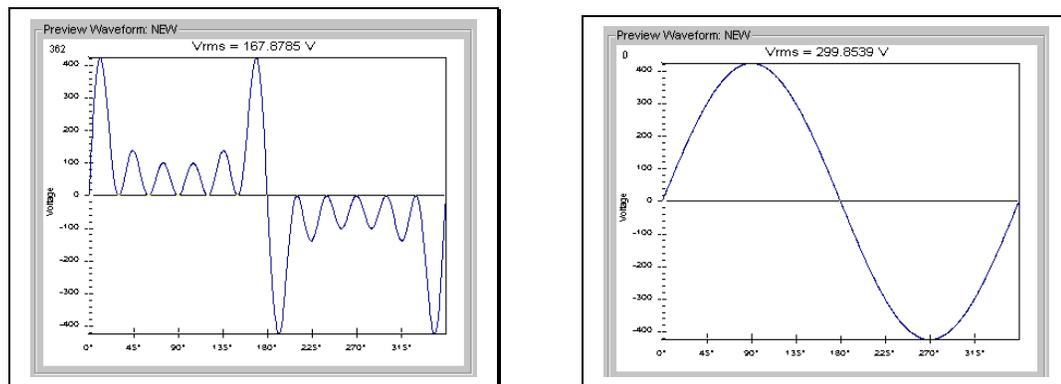
Figure 4-60: Waveform crest factor affects max. rms voltage
