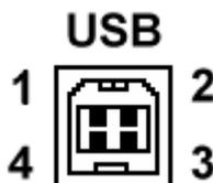
Figure 3-12: USB Connector pin orientation.
