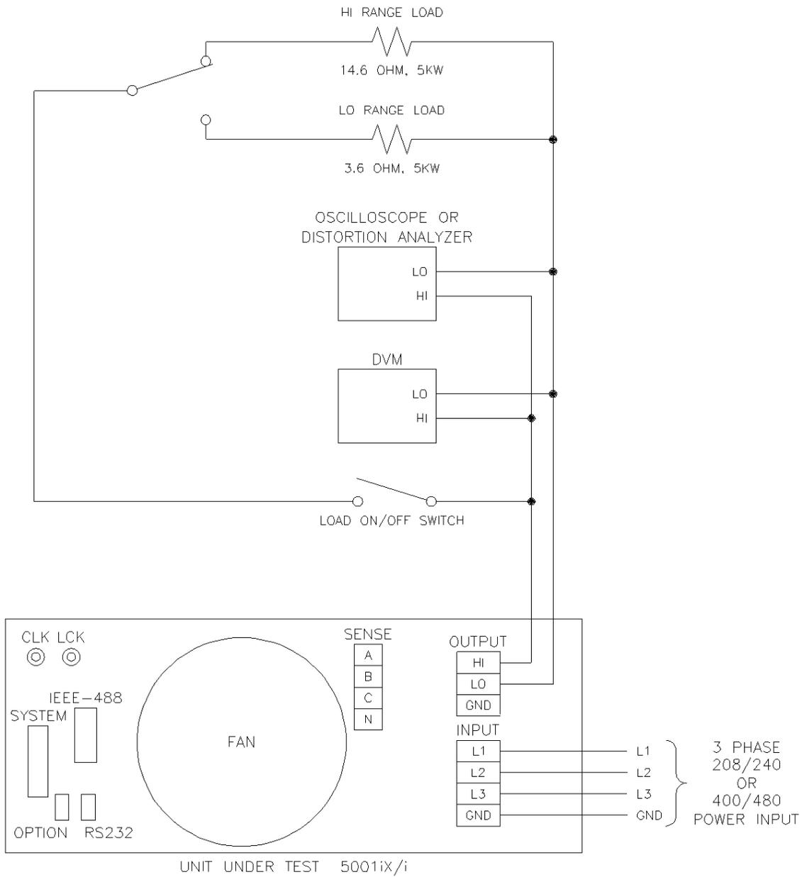
Figure 3-21: Single Phase 10000 VA System (NSG 1007-10-208/i)
