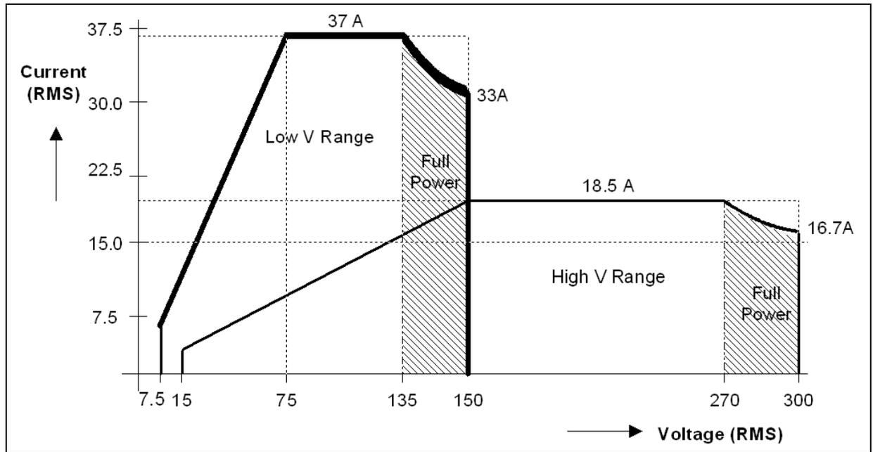
Figure 2-3: NSG 1007-5-208 / NSG 1007-15-208 - Voltage Current rating, AC mode
