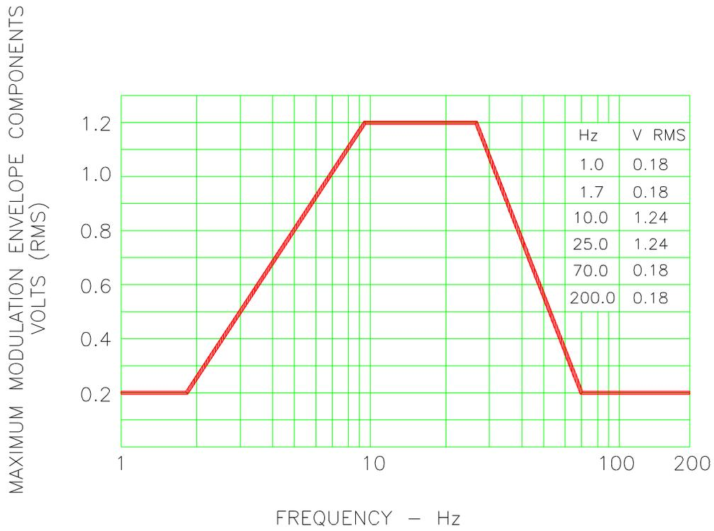
FREQUENCY CHARACTERISTICS OF AC VOLTAGE MODULATION ENVELOPE
