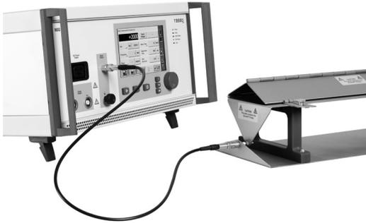
If INA 3825 accessory is used, connect the Interlock cable to the interlock input of your generator, use the INA 3825 to cover the CDN 3425 the way the interlock switch (rear side – middle) gets activated.
