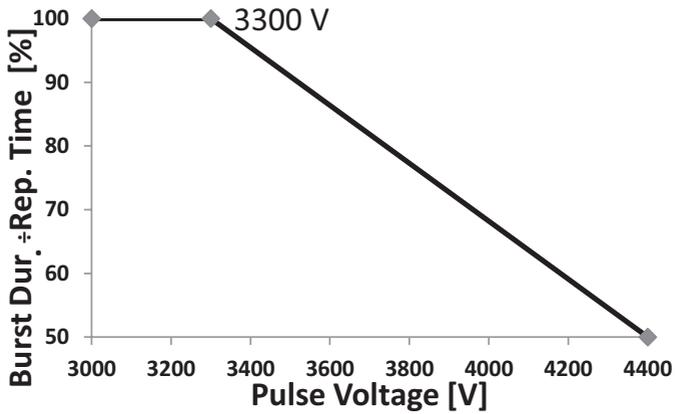
(Burst Duration ÷ Repetition Time) @ 100 kHz Pulse
