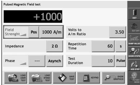
**Pulsed Magnetic Field test window**
