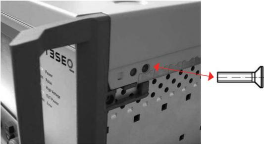
Removing the NSG 3040 side panels and cover
