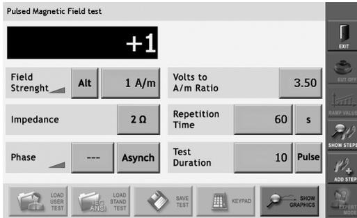
Once the right Volts to A/m ratio – which is available on the INA 752 as well then in its calibration certificate is entered in its respective field, the user will be able to enter the required test level directly in A/m – no need for him to proceed with calculations, the instrument software does the job.
