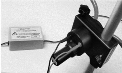
The tests are carried out using the so-called immersion method, i.e. the item under test is placed in the center of the loop. The test is performed in accordance with the IEC 61000-4-8 (mains frequency) or IEC 61000-4-9 (pulsed) standards for magnetic fields.
