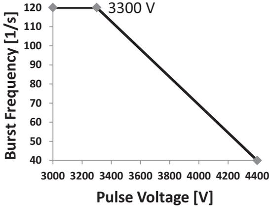
Burst frequency @ 100 kHz Pulse
