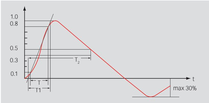
Front time  $T_1 = 1.25 \times T = 8 \mu\text{s} \pm 20\%$
