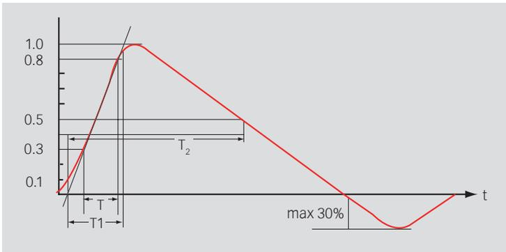
Front time  $T_1 = 1.67 \times T = 1.2 \mu\text{s} \pm 30\%$
