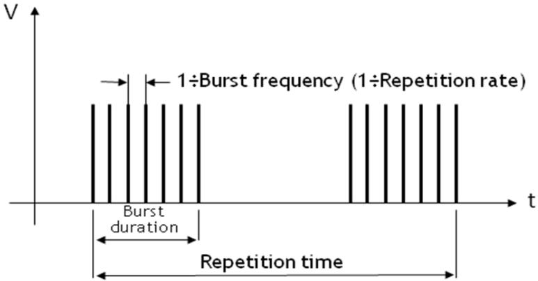
Explanation of "Burst frequency", "Burst duration" and "Repetition time" parameters
