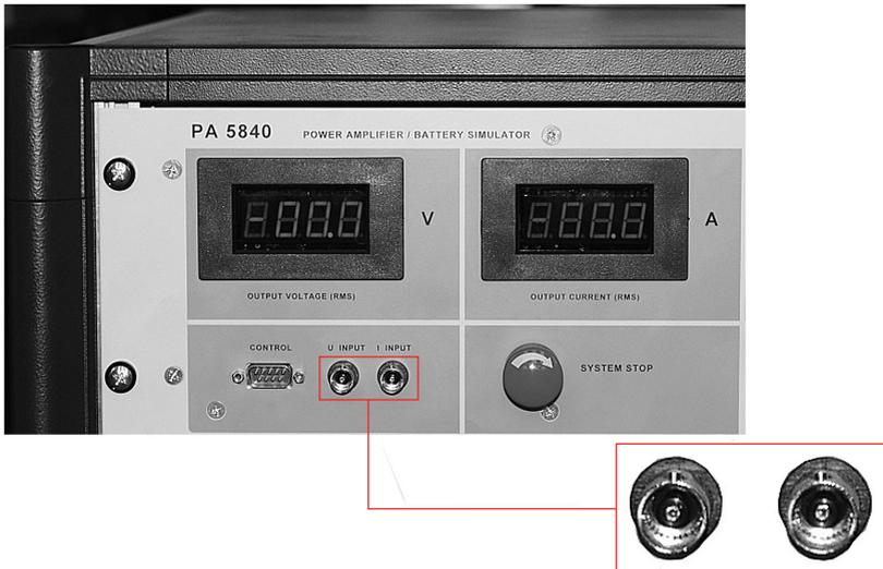
This inputs may be used in special applications when the NSG 5000 series is not used. Another function generator may be used to control the DC amplifier. 1 V input is 7 V output.
