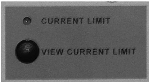
This LED indicates that the current limit has been reached. The current does not take effect until the conditions from the "CURRENT LIMITATION" field are met. Pressing the "VIEW CURRENT LIMIT" button displays the current limit on the "OUTPUT CURRENT" display.
