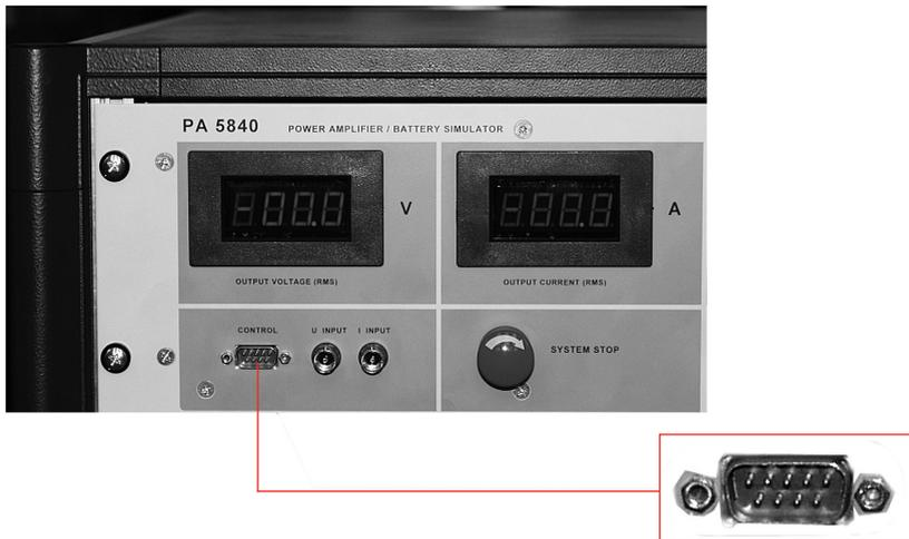
The “CONTROL” connector is an input port from the function generator card. Connect the 9-pin DSub “CONTROL” connector to the appropriate connector at the function generator card of your NSG 5000 series.
