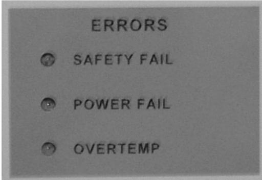
**SAFETY FAIL** This LED lights in the event of the "SYSTEM STOP" button being pressed.
