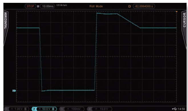
Figure 12: MIL-STD-704 Rev F, HDC 201 Cond K @ 10 mS/div – Detail
