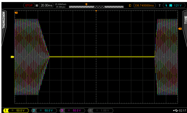
Figure 14: DO-160G Section 16.5.1.4 b Test Condition 7
