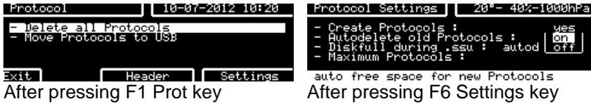
If this function is set to “on”, when a test is started, TRA3000 F-S-D-V will check there is enough memory for the new protocol. If there is insufficient memory, test protocols will be deleted starting with the oldest. TRA3000 F-S-D-V only creates sufficient space for the new protocol.
