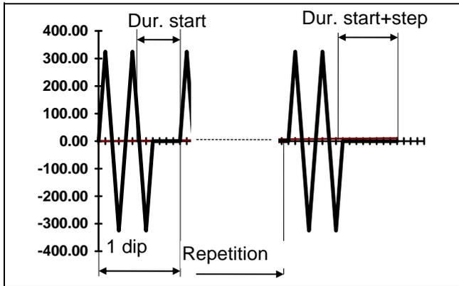
Smallest step is  $1/f$ . ( $f$ =Mains Power frequency EUT)
