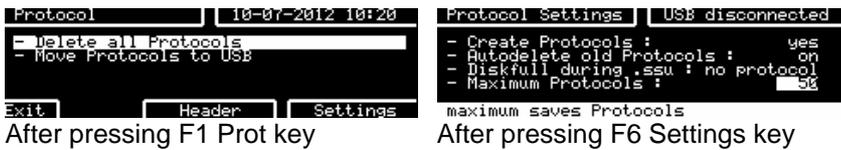
This function defines the maximum number of protocols that can be saved in TRA3000 F-S-D-V internal memory. If this value is exceeded, the oldest protocols will automatically be deleted. First-in-first-out. Default value is 50.
