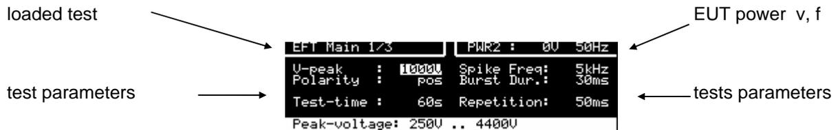
When the EDIT button has been pressed the dialogue line indicates the possible range like v, f, time, etc.
