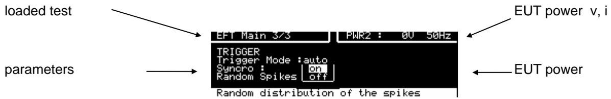
Randomly distributed spikes can drastically reduce the test time, especially for digital circuits. Weak points of EUT are found very rapidly.
