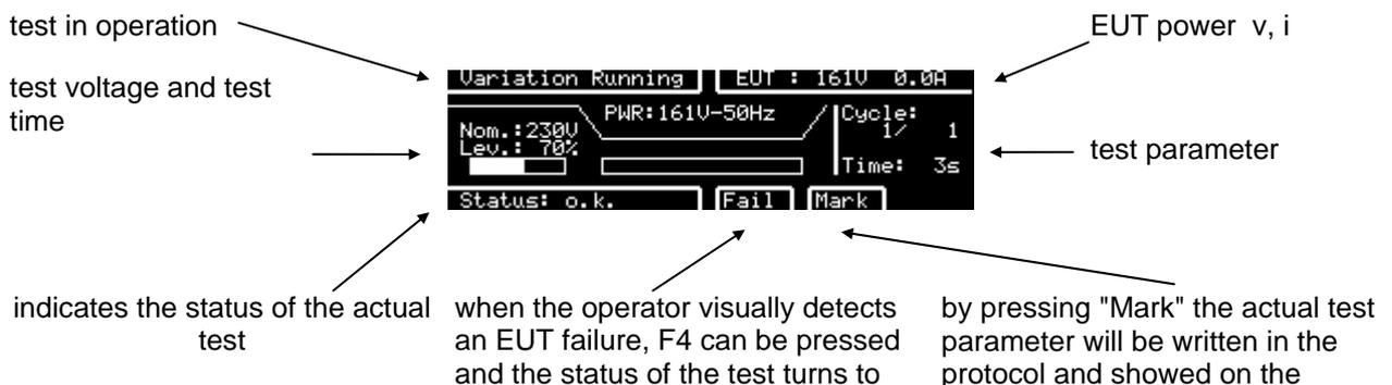
"failed". Protocol shows " test failed" display at test end.
