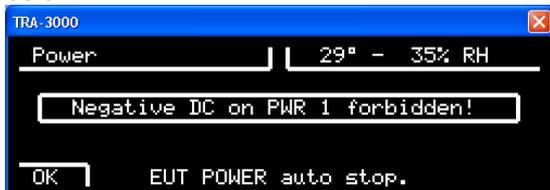
Without any guarantee from EMCP of correct operation the lower voltage limit of 20V can be extended by selecting "No" on Power 1 see display below.
