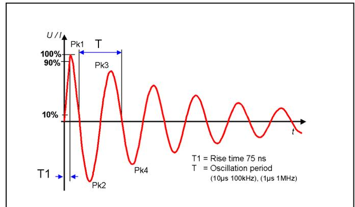
Remark: The output impedance is calculated result of the ratio of the first peak open circuit voltage and the first peak short current, measured with a 2500V pulse.
