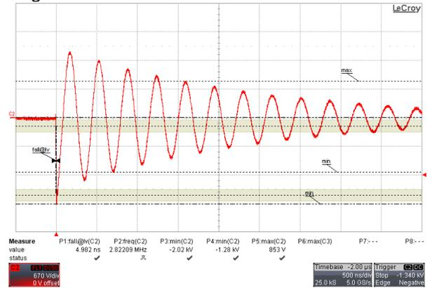
Fast Damped Oscillatory Wave, 10MHz, Coaxial output
