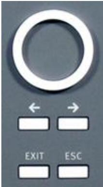
The selected parameter is blinking and can be changed by turning the knob (Inc. /Dec.). The takeover of the input value occurs after about 500ms encoder downtime. This allows the operator a brief check of the correct input value.
