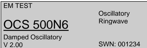
The serial number and the version number SWN are used for traceability reasons. These numbers are listed in the test reports and calibration certificates. These numbers also are listed within the test reports generated by the AMETEK CTS software ISM IEC.
