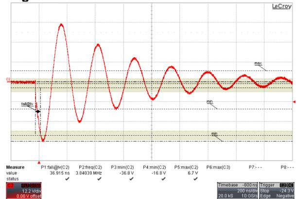
**Fast Damped Oscillatory Wave, 10MHz, Coaxial output**
