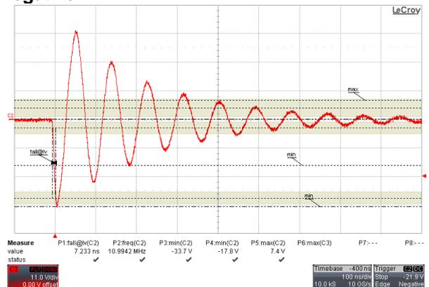
**Fast Damped Oscillatory Wave, 30 MHz, output L+N-PE**
