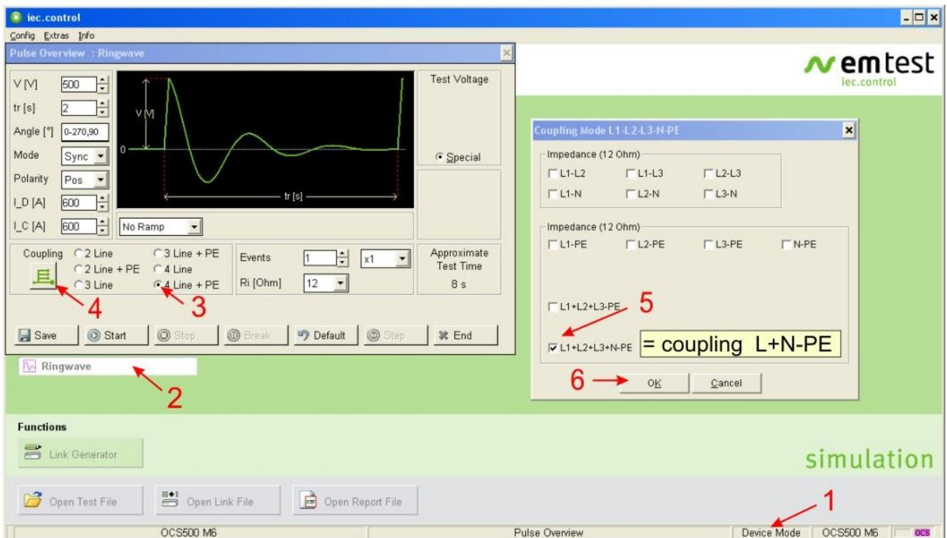
Figure 11.1: Coupling L+N-PE with software IEC.control
