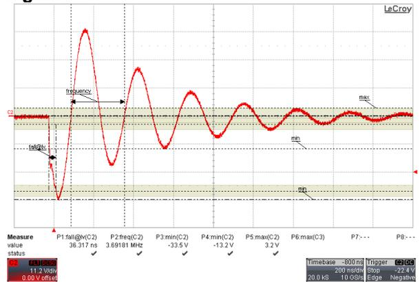
**Fast Damped Oscillatory Wave, 10 MHz, output L+N-PE**
