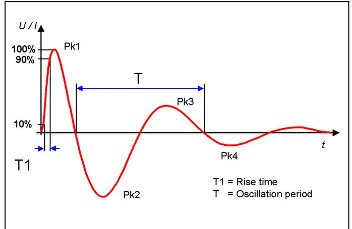
Remark: The output impedance is calculated result of the ratio of the first peak open circuit voltage and the first peak short current, measured with a 4000V pulse.
