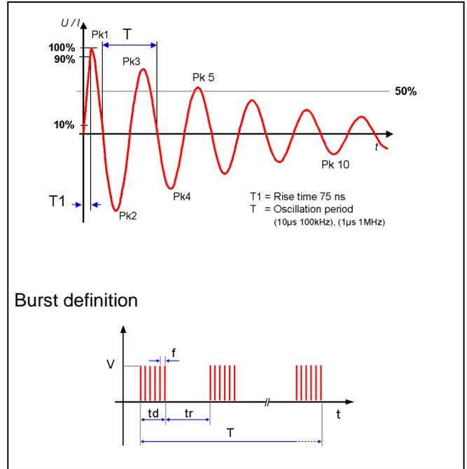
Typical pulses, measured with a calibrated equipment
