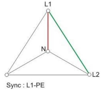
The tables below shows the correction angels considering the phase in a 3-phase system with connected L1 to the sync input. The user must set the correction angle value manually.
