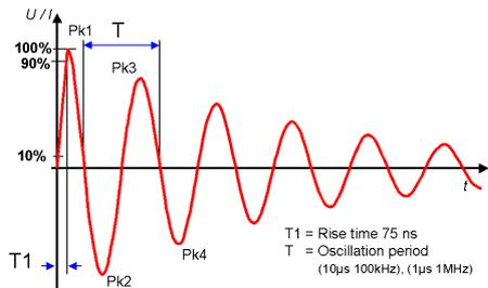
**Option required for Magnetic Field Test per IEC 61000-4-10**
