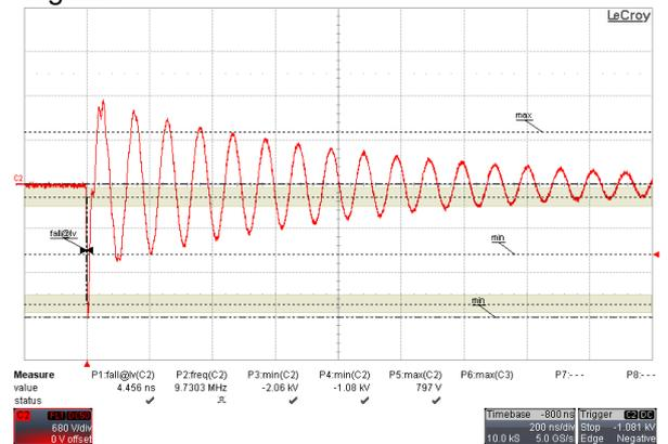
Fast Damped Oscillatory Wave, 30 MHz, Coaxial output
