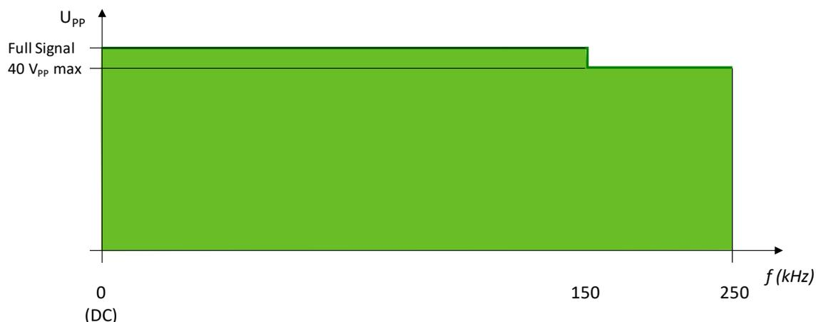
Derating at Frequency in Extended Operating Mode
