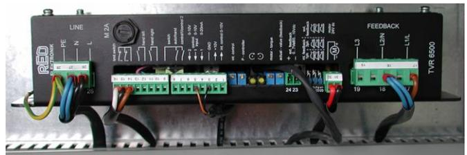
By using the additional switching function (set point 1 and set point 2), two different set points can be operated eg. hand adjusted potentiometer for set point 1 and an external control voltage from a supervisory control system for set point 2. By switching the input, set points 1 and 2 can be changed from one to the other.
