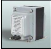
The used Solar transformer 6220-1A has a 2:1 turns ratio transformation at 1kHz. This ratio will change with higher frequencies. At 100kHz the effective ratio is more like 16:1. EM Test thinks the inter-winding capacitance results in a higher than anticipated drive voltage to produce the +/-5V signal at the secondary.
