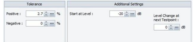
If the first measurement is already too high the user can reduce the start Level ( example to -30dB)
