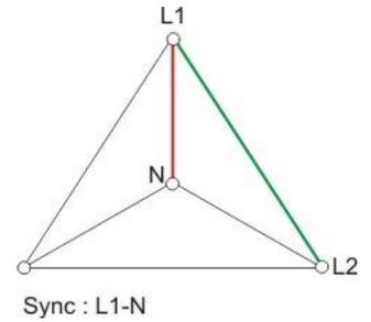
The tables below illustrate the correction angles considering the phase in a 3-phase system with synchronization signal from L1-N lines. The generator firmware will automatically add the correction angle to the settled value.
