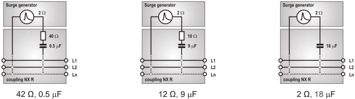
For coupling with the impedance  $42 \Omega$ ,  $0.5 \mu\text{F}$ , the coupling network PCN 7-R s-1 is required for coupling.
