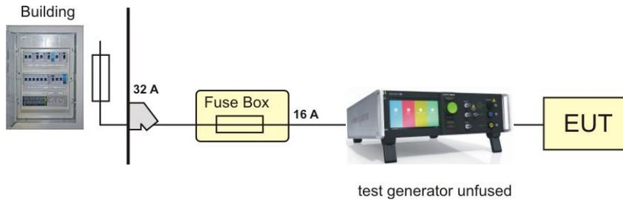
**3.4.2. EUT power ON/OFF with supply Line to Line (400V)**
