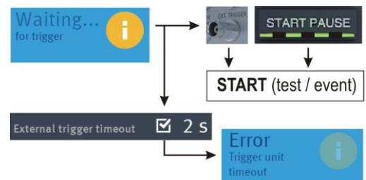
Start Trigger flowchart example from burst
