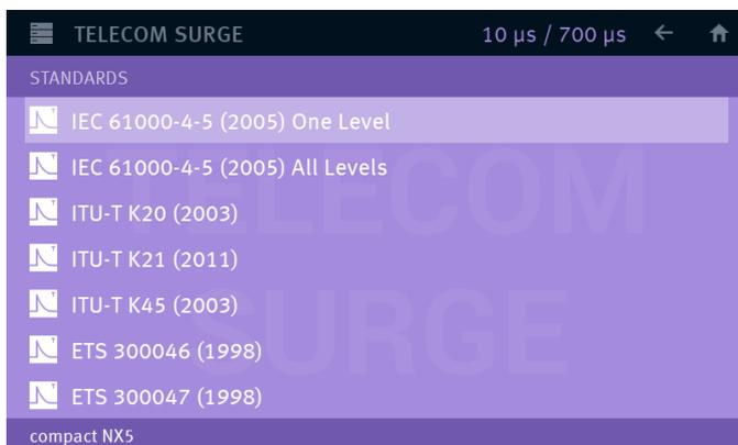
The Telecom Surge Standard menu offers a list of standards. The name of the standard defines the characteristic of the rulers that is given in the application of the standard.
