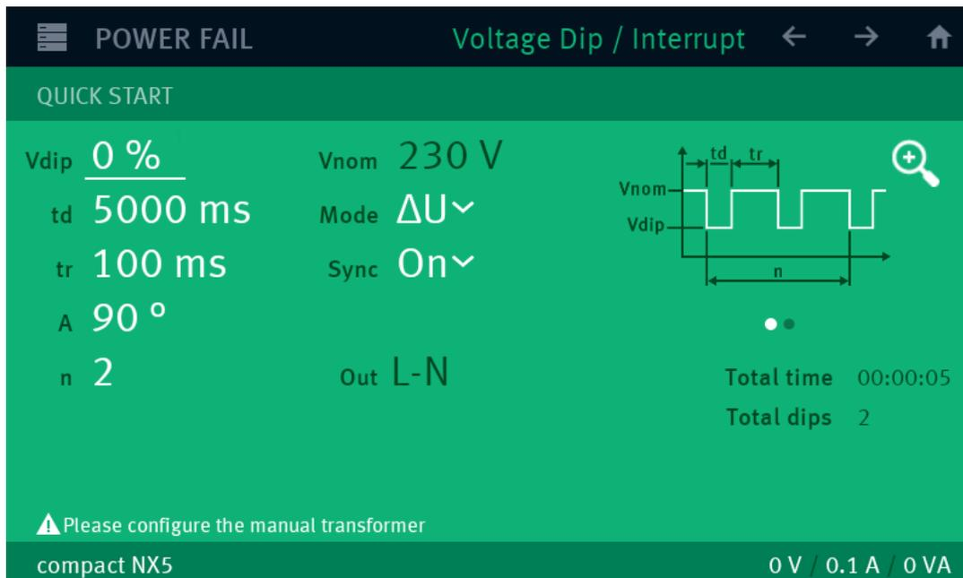
During the test the power change to PF2 for 5 seconds. During this 5 seconds the user has to connect the CA PFS to the output of the co
