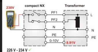
**Final screen of max. voltage adjustment**
