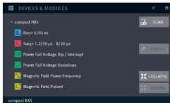
Module screen shows all recognized modules in the present system.
