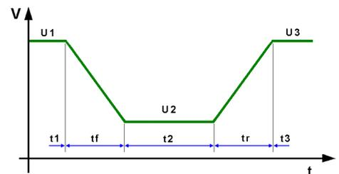
For new FDIS IEC 61000-4-11 (2004) use a new procedure for voltage variation, who simulate a voltage dip during a motor start.
