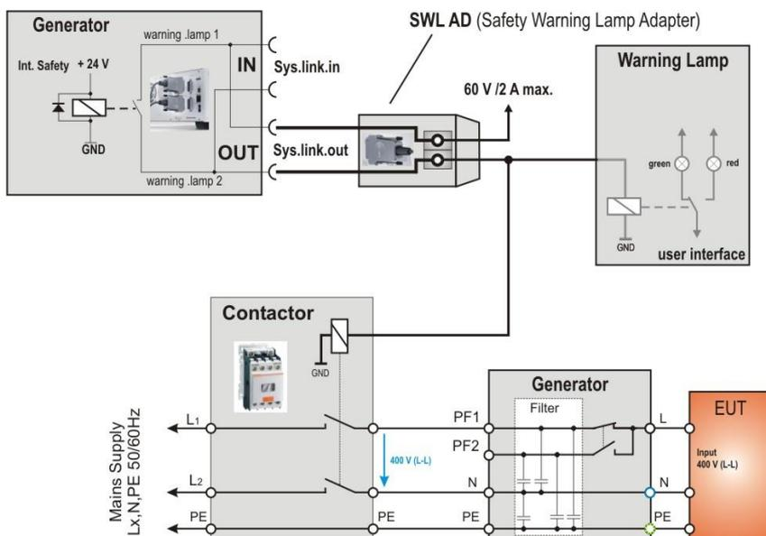
EUT power setup for a test device powered with 400 V line to line
