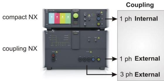
**Internal** Pulse output at the **compact NX5 CDN** - 1 phase
