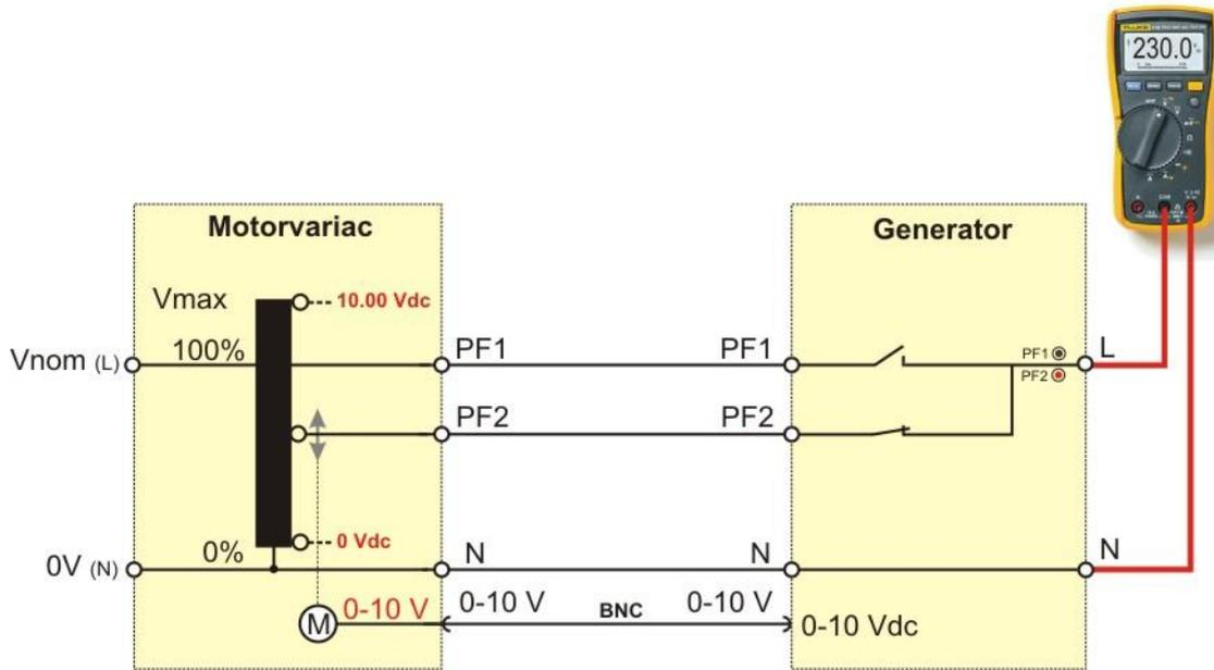
Setup for adjust the external voltage variac to the compact NX
