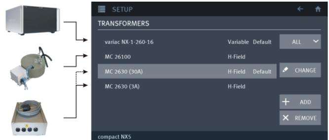
Note: The MC 2630 has two ranges and therefore the NX generator list this current-transformer in the configuration for (1 A) and (30 A) range. Set the range switch of the MC 2630 to the correct position before starting the test.
