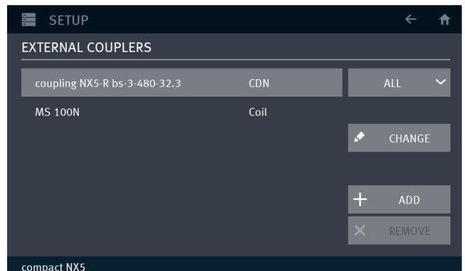
**Long click** to **coupling NX 5-R bs....** will enable the settings to CDN parameters. **Serial number** and **Firmware version** are indicated (factory setting)
