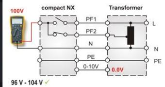
**Check at Vnom (0 V) level at zero position**
