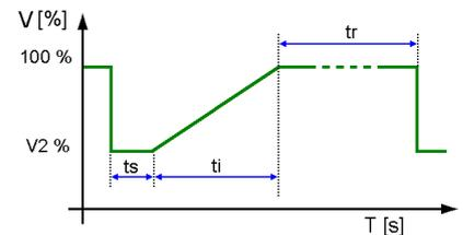
The speed of the voltage variation depends on the max. speed of the motorvariatic and the control setting of the integral action controller. The behavior can be influenced by the parameter  $V_{nominal}$ . Setting in the setup menu Setup / F5 Voltage setting.
