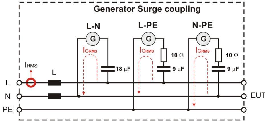
**Current in the coupling path measured by the EUT current meter**
