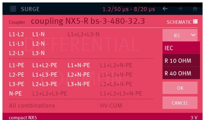
Example with setting of railway coupling 42 Ω, 0.5 μF for DC application.
