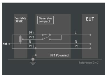
**NOTE:** PF1 is the default setting for general application for Burst, Surge and Power Fail testing.
