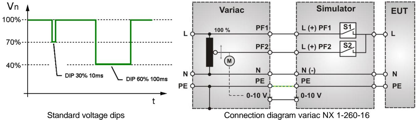
The unit has to be connected at the rear part of the equipment. For connection safety labor cables shall be used.
