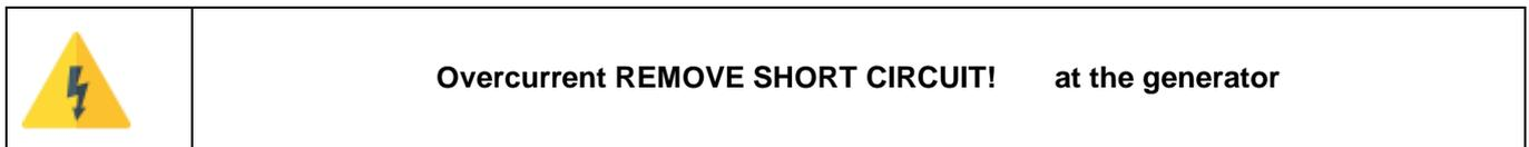
This error message appears after a short circuit at the EUT output plugs. This current can be up to 700A during few  $\mu$ s and will be detect from the overcurrent detection.
