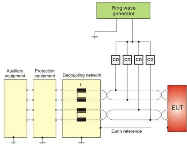
**Example: Coupling to symmetrical unshielded high-speed data lines**
