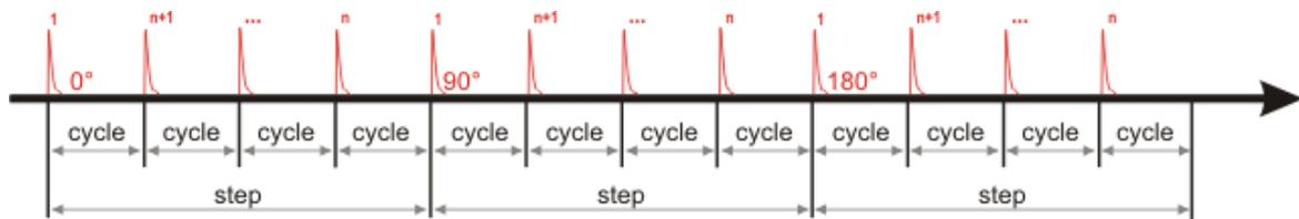
Example with voltage iteration that illustrate trigger out for cycle and step
