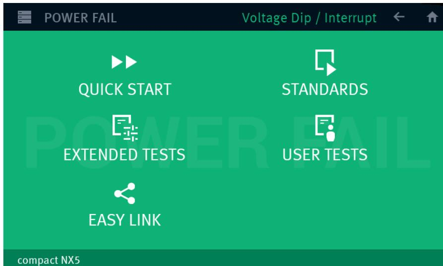
Main Menu Power Fail for voltage dips and interrupt tests
