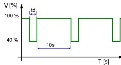
As long as the external transformer variac NX 1-260-16 is used, controlled by an analogue 0-10V control voltage, the test is conducted automatically. If this option is not available the manual test routine shall be used.
