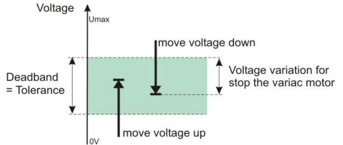
The following procedure will guide the user through the Set Voltage procedure. The setting procedure for Vmax and Vnom is listed in the figures below.
