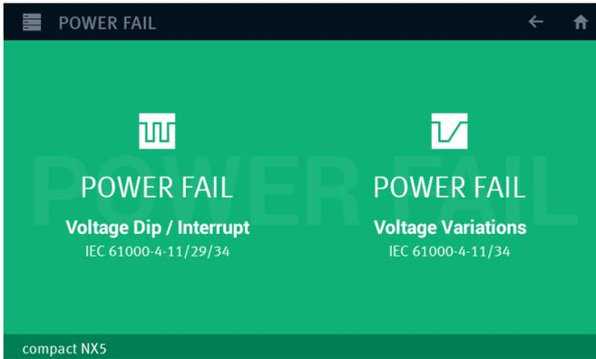
Main Menu Power Fail for voltage dips and interrupt tests and voltage variation
