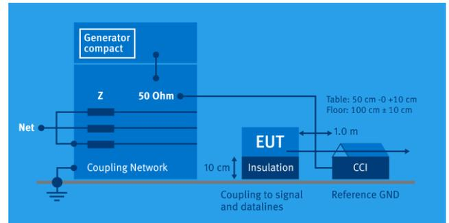
The distance between any coupling devices and the EUT shall be  $(0.5 - 0/+0,1)$  m for tabletop equipment testing, and  $(1,0 \pm 0,1)$  m for floor standing equipment, unless otherwise specified in product standards. When it is not physically possible to apply the distances mentioned above, other distances can be used and shall be recorded in the test report.
