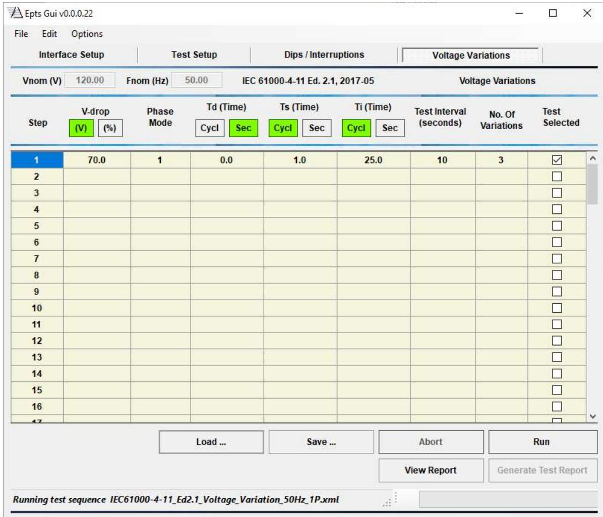
The screenshot shows the EPTS GUI interface for the Voltage Variations test. The window title is "Epts Gui v0.0.0.22". The menu bar includes "File", "Edit", and "Options". The main interface has tabs for "Interface Setup", "Test Setup", "Dips / Interruptions", and "Voltage Variations".
