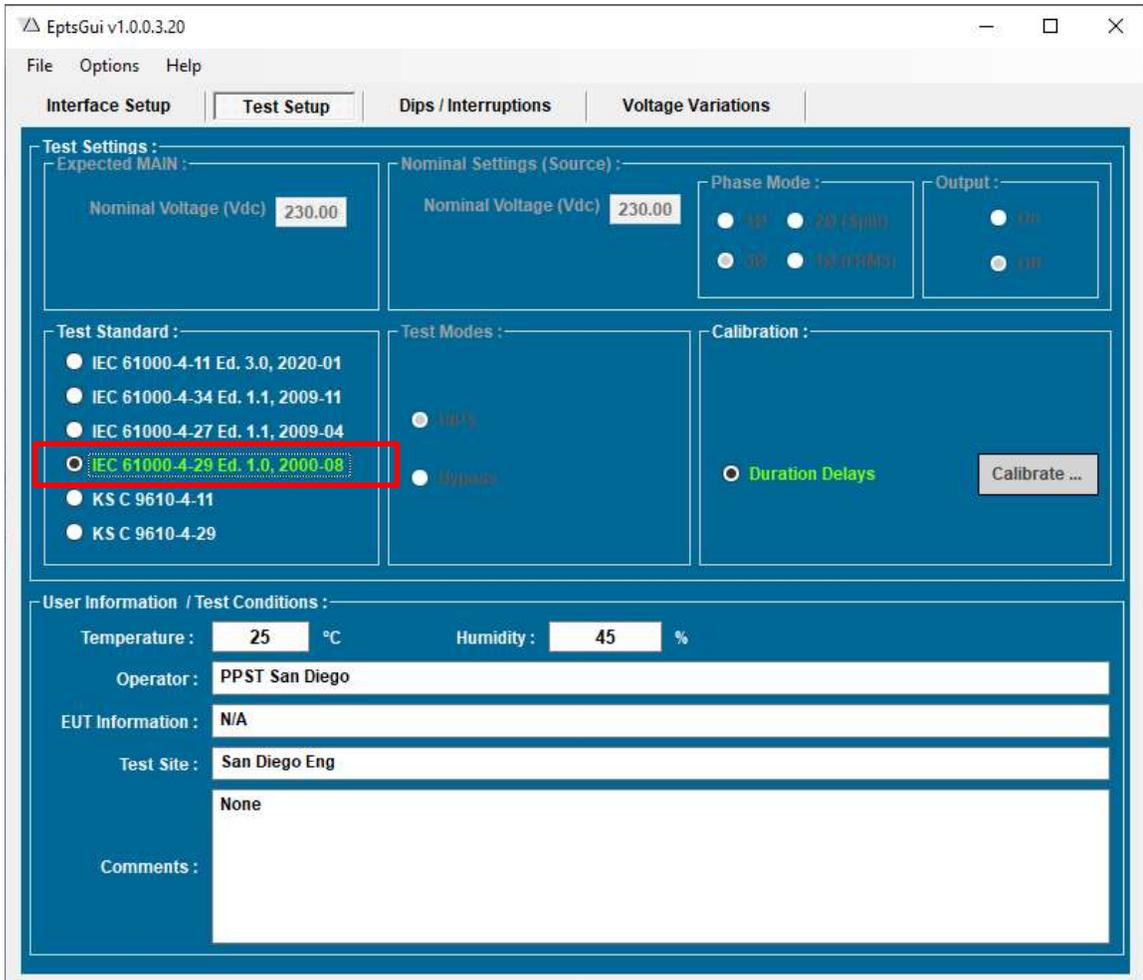
Figure 8-1: IEC 61000-4-29 DC Test Setup Selection Screen
