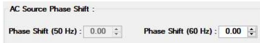
The AC power source is synchronized to phase A of the AC Mains input side of the EPTS and it is imperative that the phase difference between the Mains Phase A (L1) L-N voltage and the AC power source output in SYNCED mode is as close to zero degrees as possible. (zero phase shift between the two. This requires the use of a two channel digital scope.
