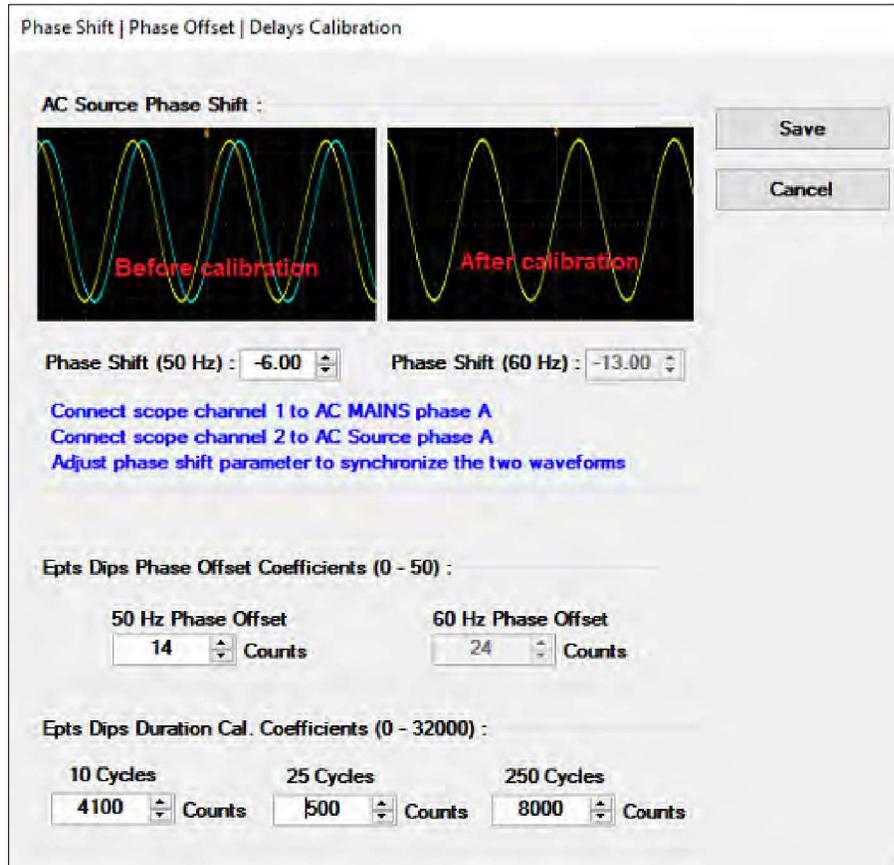
There are sync offset calibration coefficients for both 50Hz and 60Hz Mains applications. Make sure you adjust the coefficient for the correct Mains frequency.
