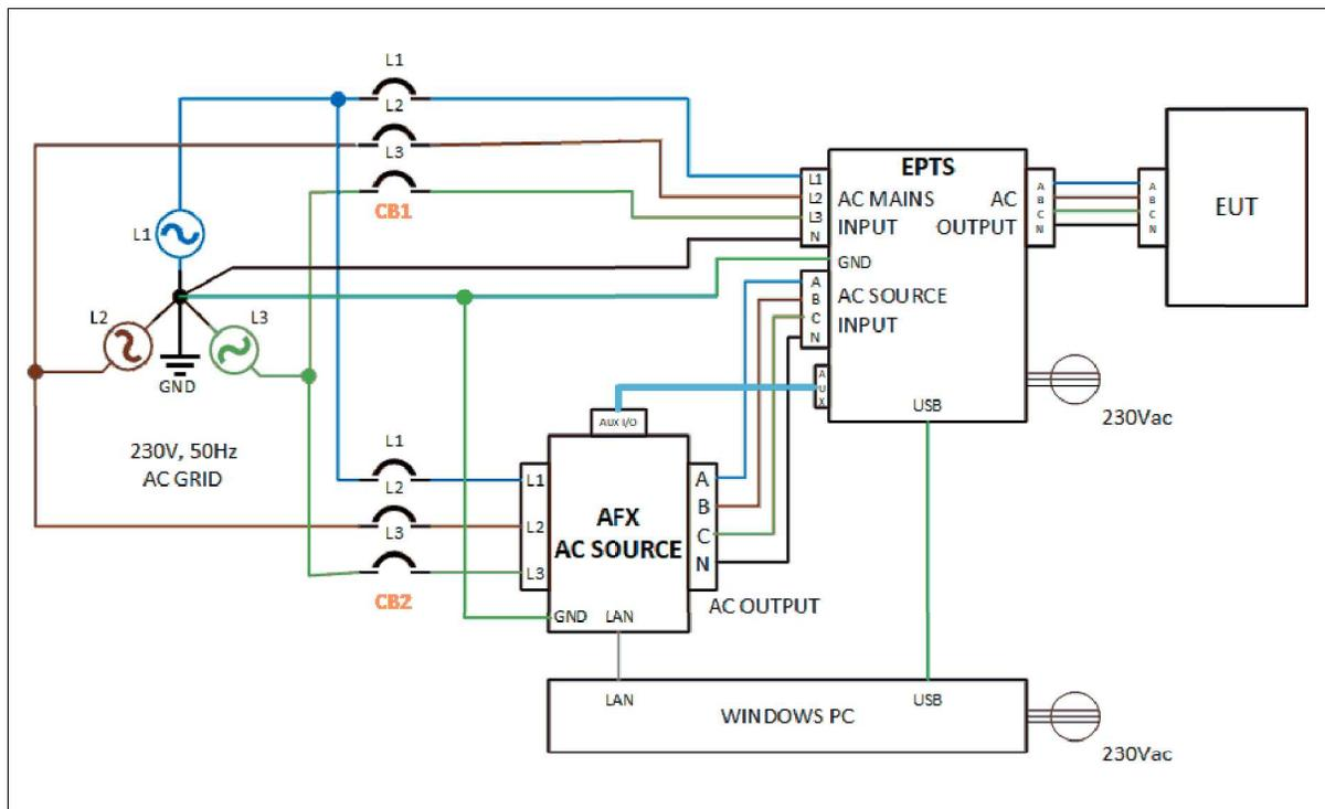
Figure 5-3: EPTS System Schematic for AC Test Mode
