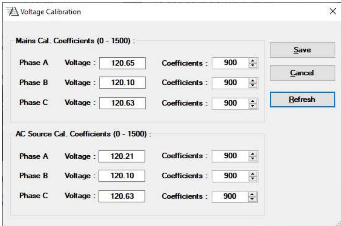
3. For each available Mains input phase, measure the Phase Line to Neutral voltage using the DMM. The expected voltage should match the actual Mains voltage at your location.
