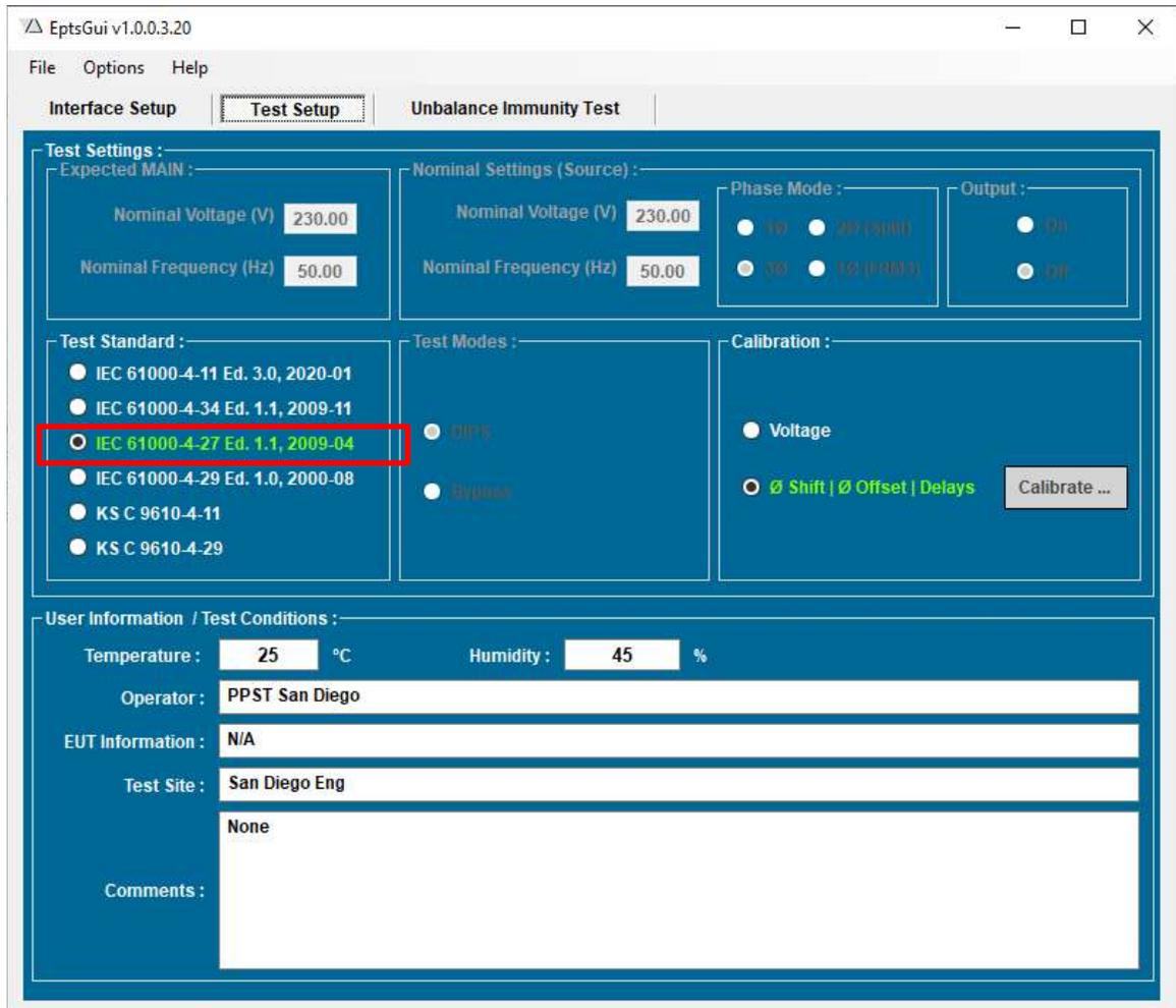
Figure 7-1: IEC 61000-4-27 DC Test Setup Selection Screen
