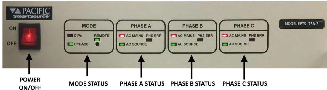
1. Power On/Off Switch. Turns internal control circuits on or off.
