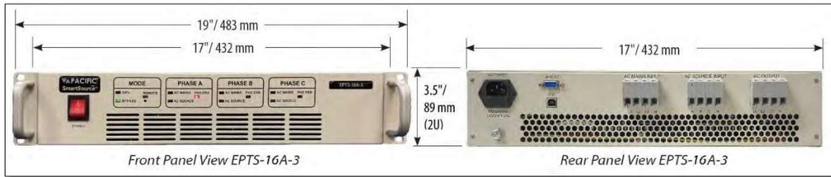
Figure 4-1: Dimension Drawing EPTS Module Series 2U Models 16A
