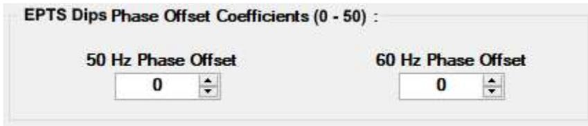
These two calibration coefficients are used to provide optimal phase angle drop positions for either 50Hz or 60Hz testing. Each frequency mode has its own independent coefficient. This calibration was performed at the factory and the calibration file provided with the EPTS must be copied to the user's PC so the correct coefficients are loaded when the EptsGui is opened.
