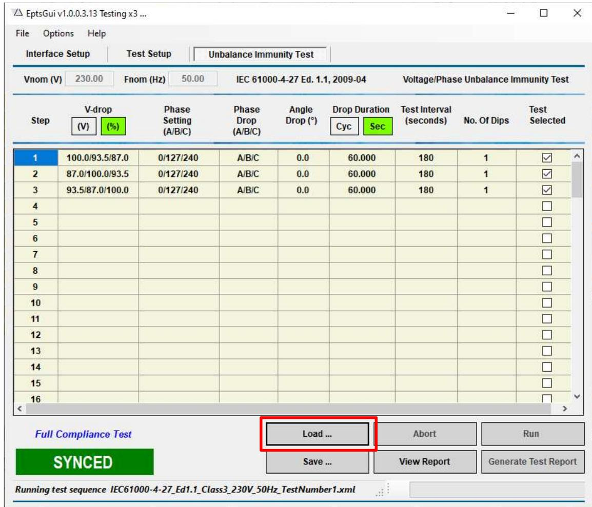
Figure 7-2: IEC 61000-4-27 Voltage Unbalance Screen
