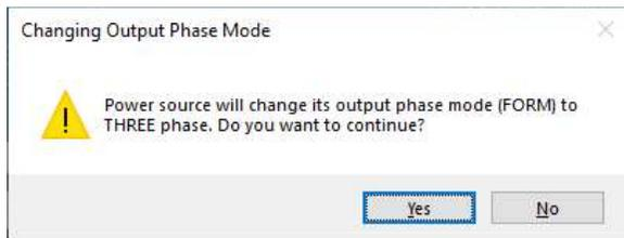
This allows the operator to check the output wiring to the load to make sure the correct phase mode and load wiring is in place. If not, click on **No** to abort. If it is, click **Yes** to proceed.
