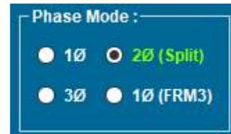
It is also important to remember that the Line to Line output voltage is 2x the L to N voltage settings on phases A and B when the default split phase angle of 180° is set. Thus, the Nominal test voltage for split phase mode when the AC line voltage is still 220Vac or 230Vac but the AMX/LMX will set each phase output to 110Vac or 115Vac to produce the required phase A to B ac voltage.
