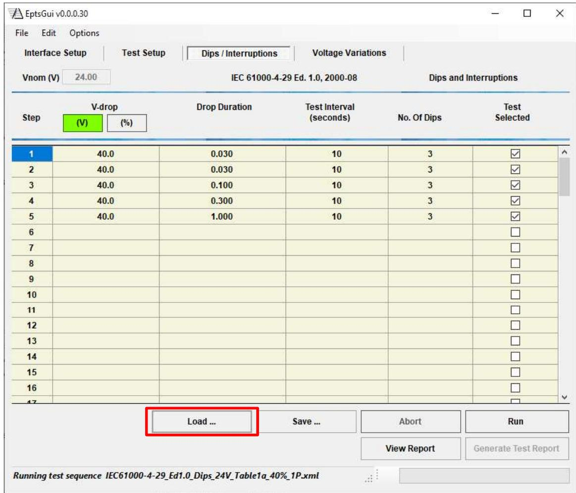
Figure 8-2: IEC 61000-4-29 Voltage Dips & Interruptions Screen
