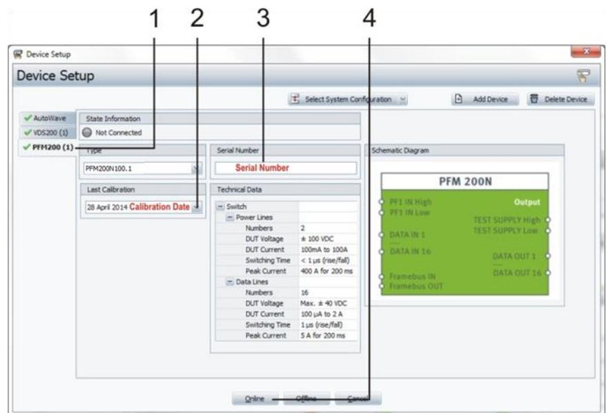
Figure 3.15: Device Setup for PFM 200N100.1
