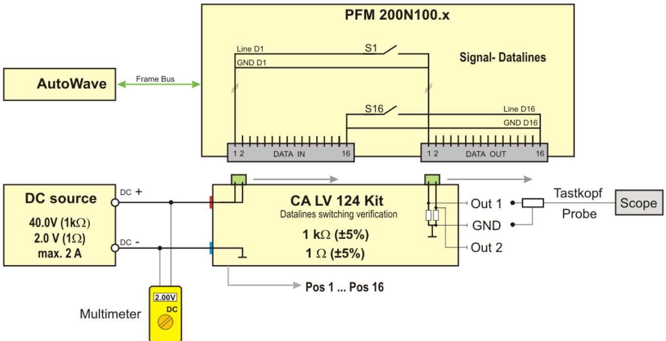
Figure 9.8: Test Setup for Reference Measurement using  $1\text{ k}\Omega$  and  $1\ \Omega$
