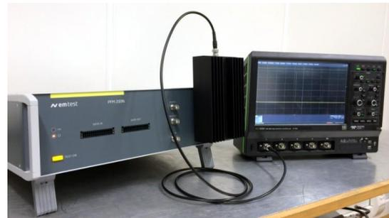
Figure 7.15: Example Verification setup with PFM 200N100.1, CA LV124-P1R and Scope
