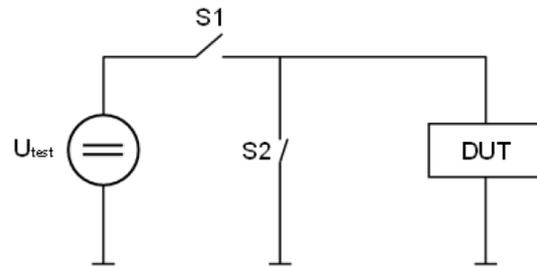
Figure 7.1: Block Diagram of E-10 Short Interrupts (LV 124)
