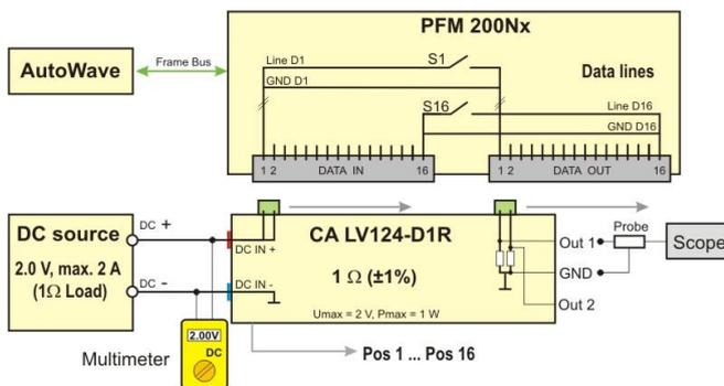
Figure 8.13: Test setup Verification schematic
