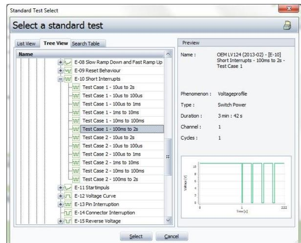
Figure 6.2: Standard List for LV 124 Test Case 1 & 2
