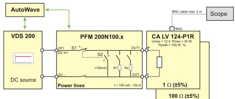
Figure 7.2: Test Setup Using EM TEST Generators
