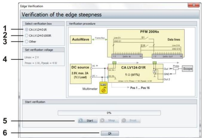
Figure 8.10: Reference Measurement Test Window
