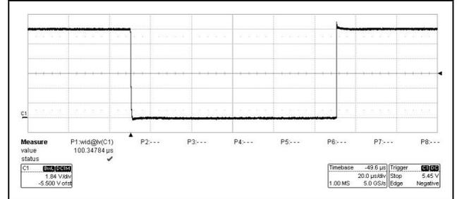
Figure 8.16: Reference measurement load 1000 Ω
