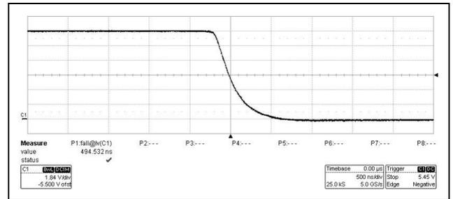
Figure 8.20: Reference measurement load 1000 Ω
