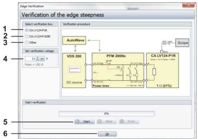
Figure 7.11: Reference Measurement Test Window
