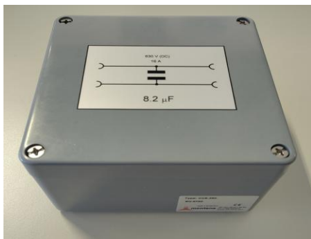
Decoupling capacitor 8.2µF for spikes test
