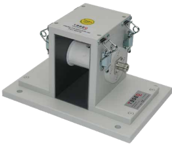
PCJ 9201B calibration jig, recommended for MD 4070 calibration
